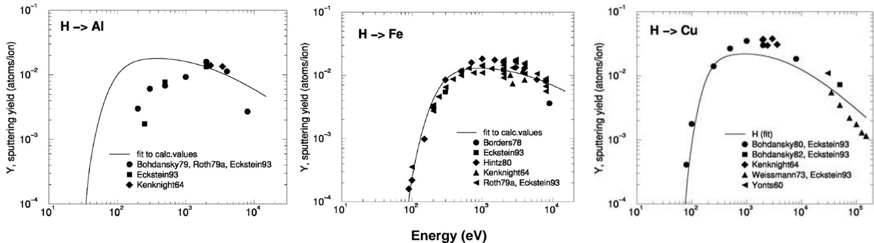
Sputtering rates of Hydrogen Atoms onto selected materials [Sputtering by Particle Bombardment Topics in Applied Physics, 2007, Volume 110/2007, 33-187, DOI: 10.1007/978-3-540-44502-9\_3]
