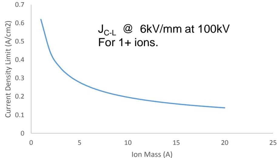
Assuming the same extraction conditions, Higher mass and higher charge lead to LESS particle current. Note this is assuming all the particles are in 1 charge state.
