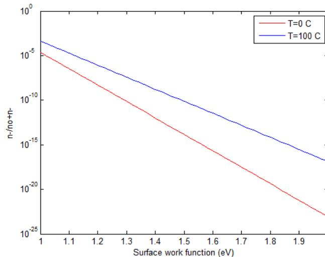
The plot shows the production probability for negative hydrogen, relative to neutral hydrogen, from a low work function surface.
