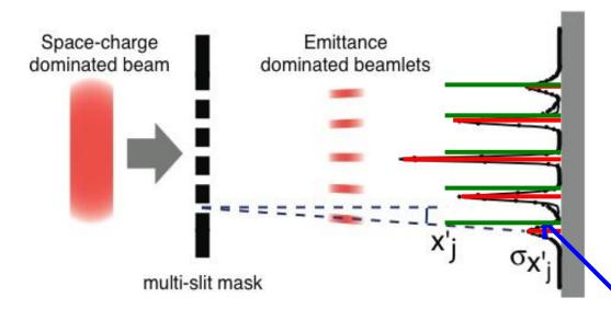
To measure the emittance for a space charge dominated beam the used technique is the well known 1-D pepperpot
