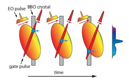
The short gate pulse overlaps with different temporal slices of the EO pulse at different spatial positions of the BBO crystal. Thus the temporal modulation of the EO pulse is transferred to spatial distribution of the SHG light.
