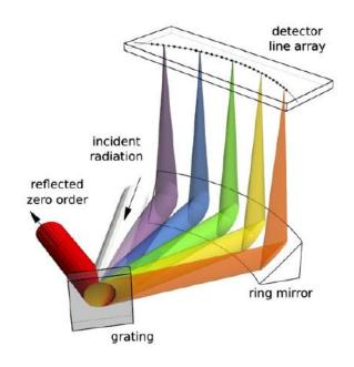
Pyro-electric line detector 30 channels @ room temperature no window, works in vacuum fast read out sensitivity
