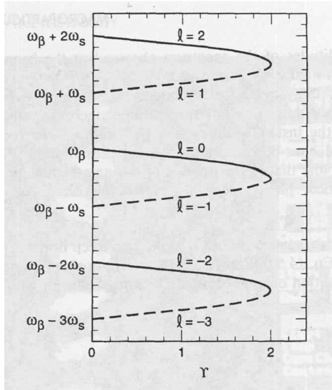
Solid curves are the spectrum of the + mode; dashed curves are that of the - mode. Instability occurs at the point where the mode frequencies merge.
