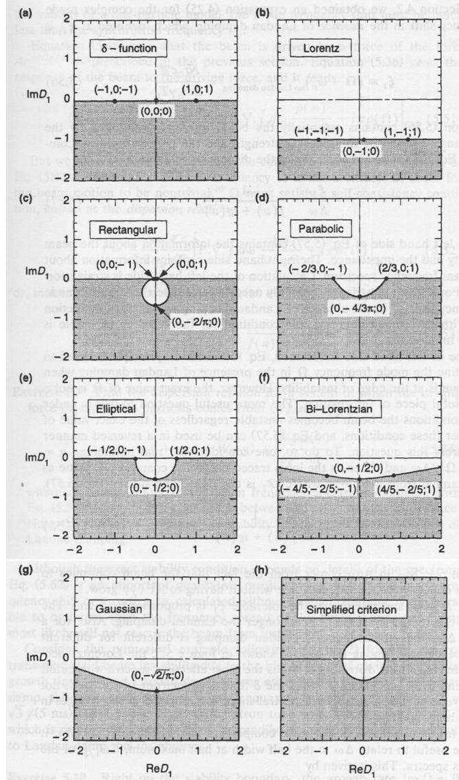
The stability boundary diagrams for various spectra. Shaded regions are unstable. The coordinates labeled refer to  $(\text{Re}\mathcal{D}_1, \text{Im}\mathcal{D}_1; u)$ . The value of  $u$  can be used to obtain  $\Omega$ . (a)  $\delta$ -function spectrum, no Landau damping. (h) is the simplified criterion (18).
