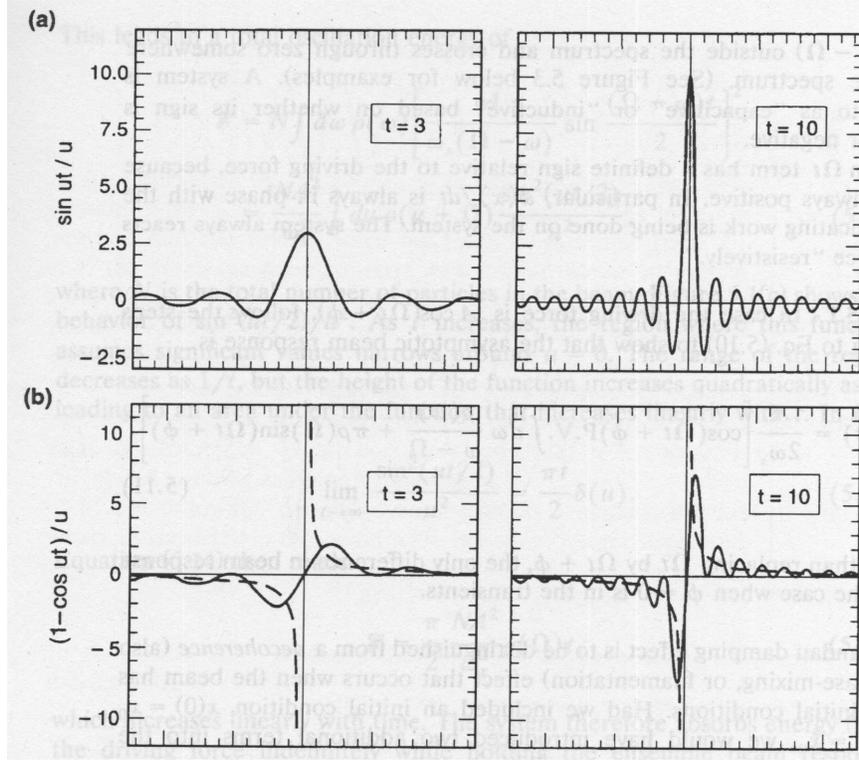
The functions  $\sin(ut)/u$ ,  $(1 - \cos ut)/u$  are shown in (a), (b) for two values  $t = 3$  and  $10$ . The dashed curves in (b) are for the function  $1/u$ . The sole function of  $(1 - \cos u)$  in (b) is to suppress the singularity at  $u = 0$ .
