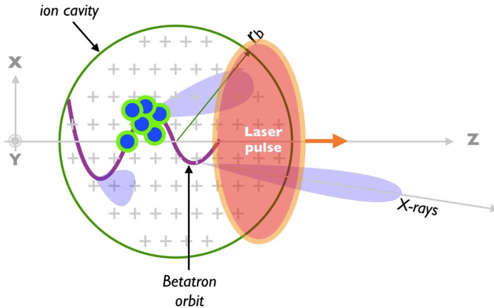
The electron, is accelerated and wiggled in the ion cavity
