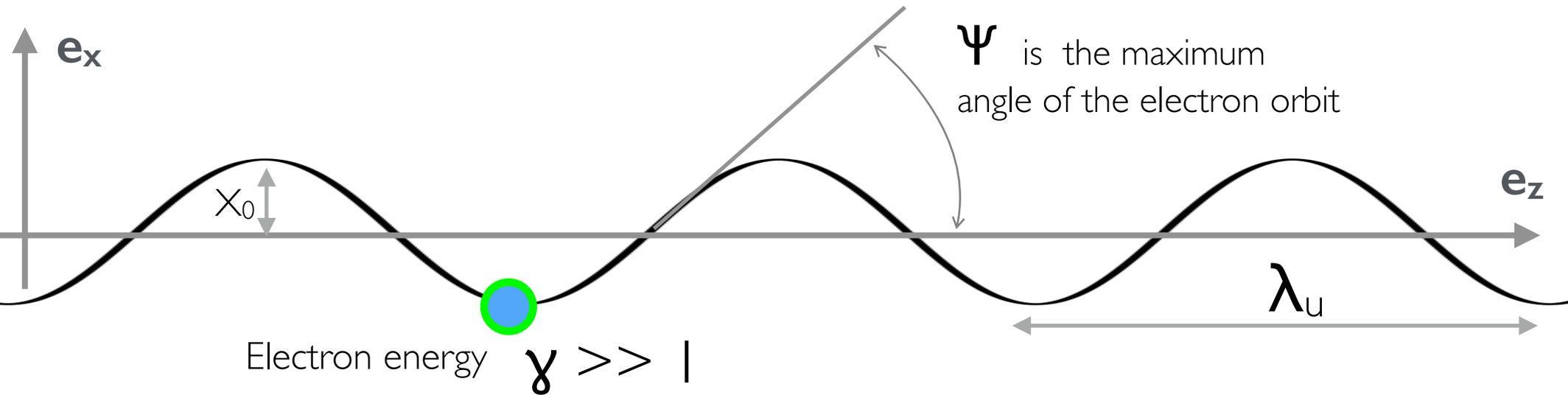
→ Relevant parameters to obtain the features of the radiation are :
