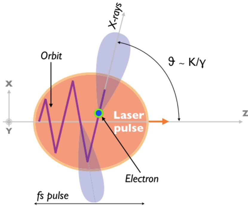
The electron, initially at rest is submitted to the EM laser field.
