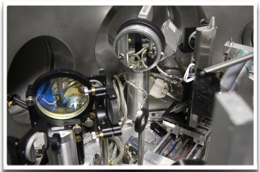
Hot electrons from laser solid interaction ionize inner shell atoms. Inner shell vacancy is filled by outer shell. This results in the emission of a short x-ray pulse
