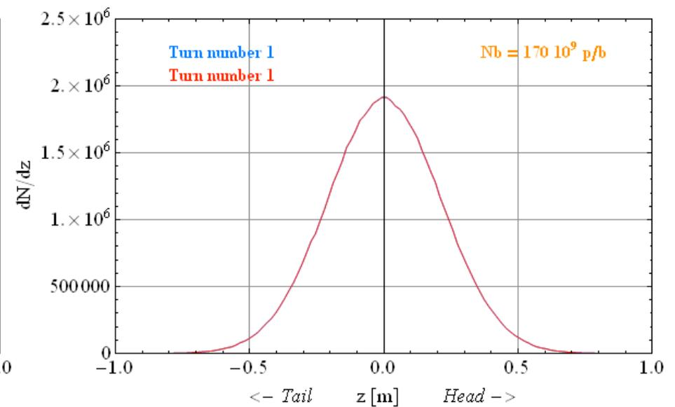
Bunch shape evolution in the regime of **bunch lengthening** ( $10^{11}$  ppb, left movie) and just above the threshold for **microwave instability** ( $1.7 \times 10^{11}$  ppb, right movie)
