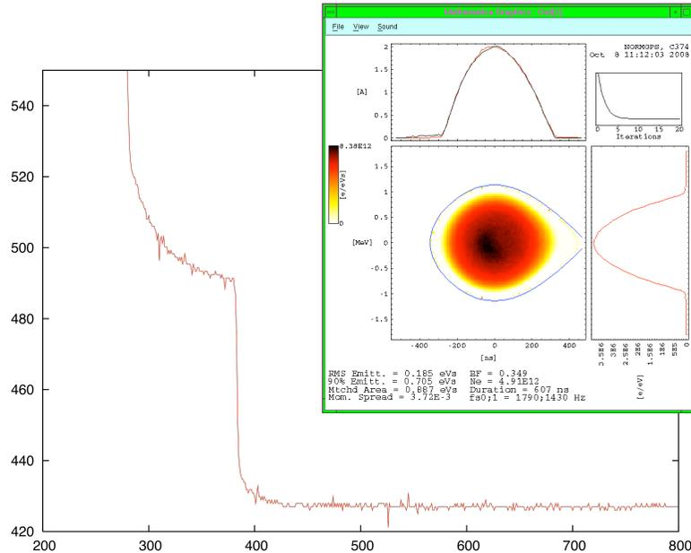
Beam loss as measured by a Beam Current Transformer
