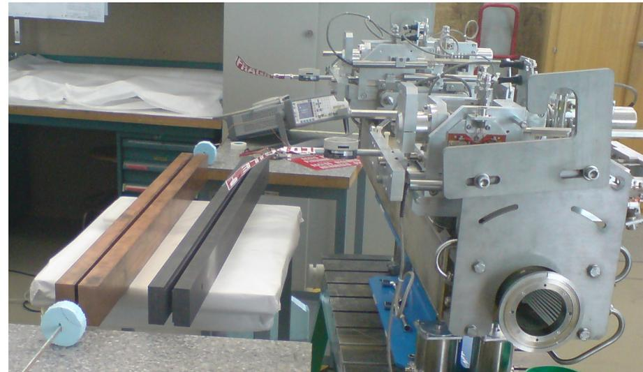
LHC collimator prototypes in copper and graphite
