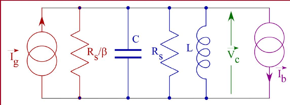
The beam current is represented by the phasor  $I_b$  at the frequency of the RF source, while the external RF source is represented by a current generator  $I_g$  whose amplitude is related to the power of the forward wave launched on the transmission line.
