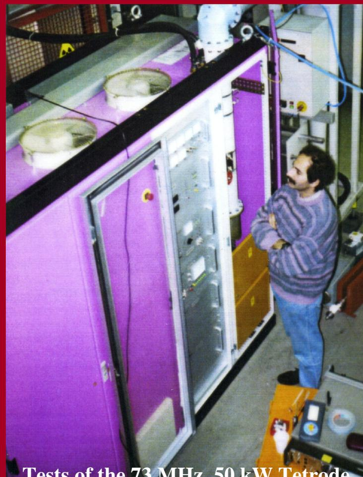
Tests of the 73 MHz, 50 kW Tetrode Amplifier for the DAFNE damping ring
