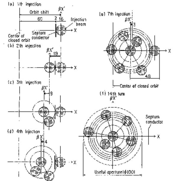
Figure: 2 Injection process in phase space at the septum conductor. (Unit ; mm)
