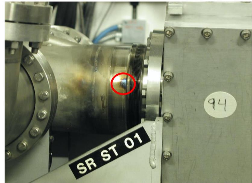
Un-controlled convoy electron burn spot at PSR, due to ~85 W of electron power.
