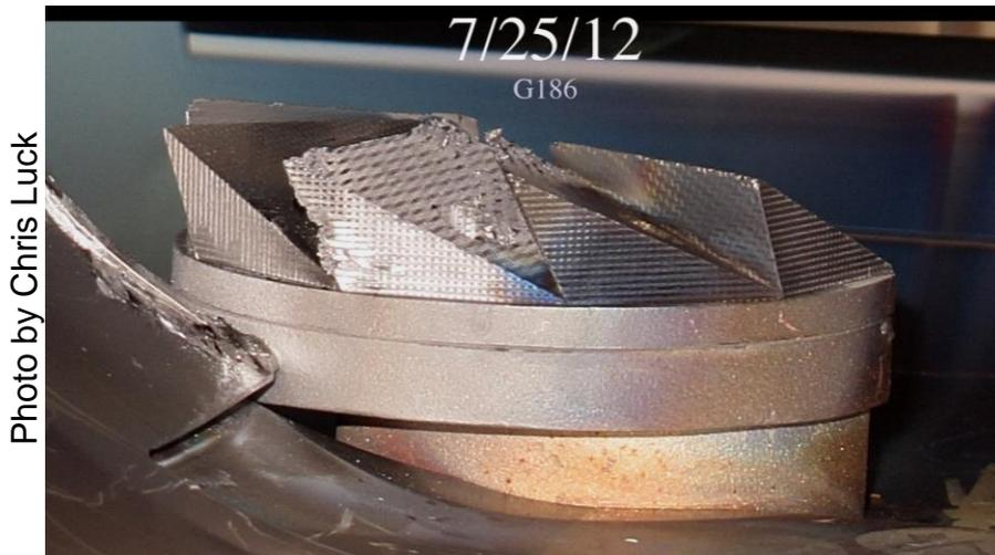
The convoy electrons are ideally trapped by this electron catcher mounted in the bottom of the vacuum chamber
