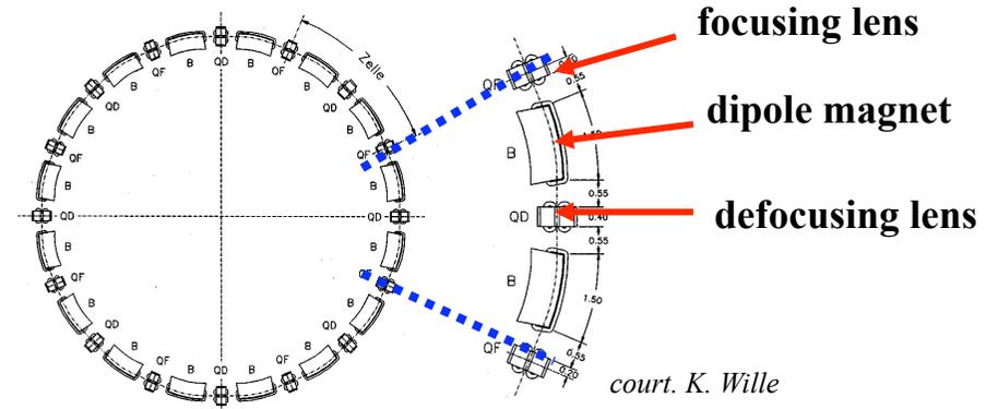
in each accelerator element the particle trajectory corresponds to the movement of a harmonic oscillator ,,
