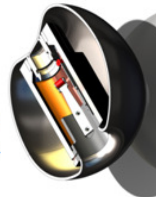
Cut-out of ball cathode design
