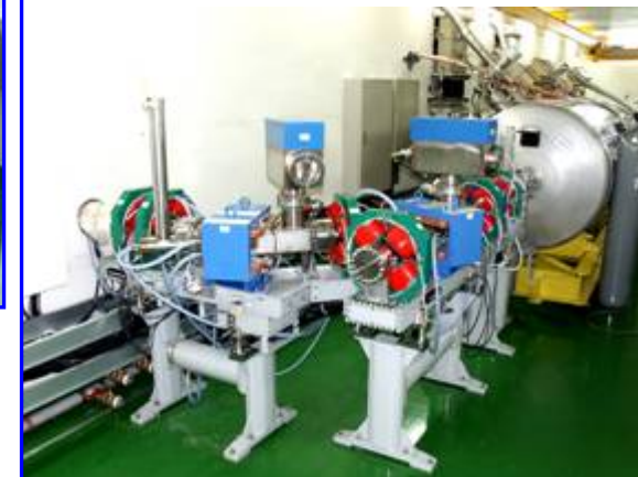
Extraction beamline 10 MeV, I_{\text{averaged}} = 5 \text{ mA}
