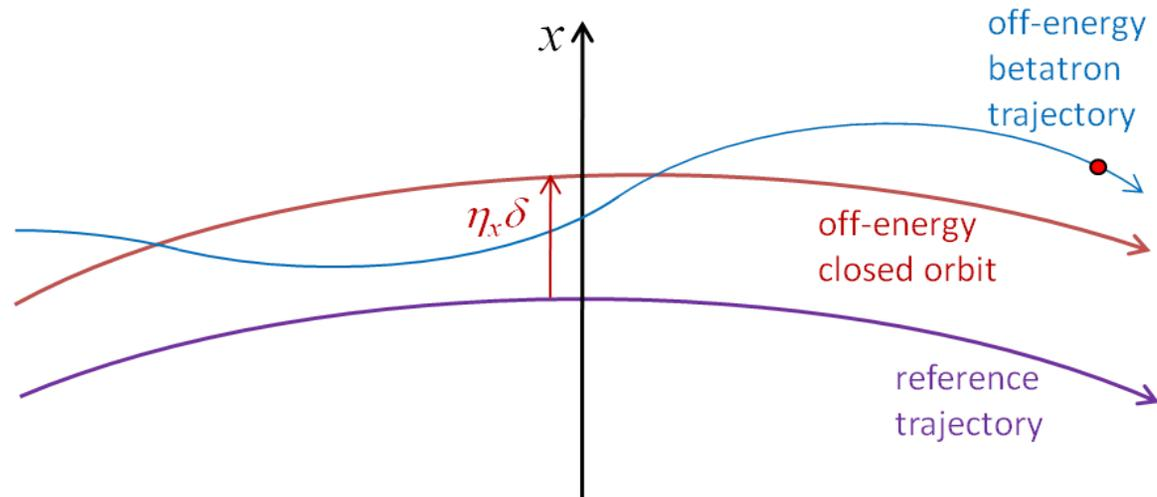
Coupling between transverse and longitudinal planes in a beam line is usually represented by the dispersion,  $\eta_x$ .
