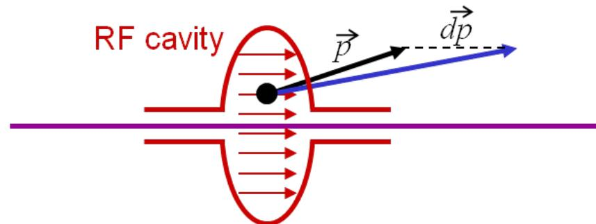
Fortunately, RF cavities are usually designed to provide a longitudinal electric field.
