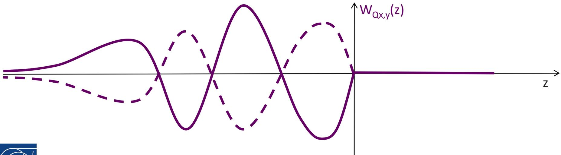
$$W_{D_x}(z) = -\frac{E_0}{q_1 q_2} \frac{\Delta x'_2}{\Delta x_1} \quad W_{Q_x}(z) = -\frac{E_0}{q_1 q_2} \frac{\Delta x'_2}{\Delta x_2}$$
