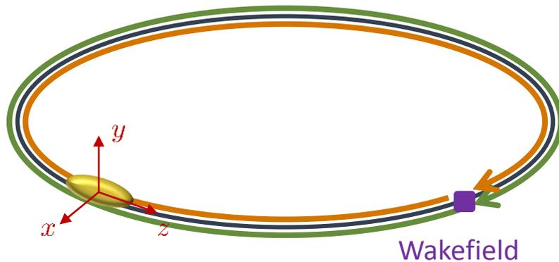
$$\begin{aligned} \left. \begin{pmatrix} x_i \\ x'_i \end{pmatrix} \right|_{k+1} &= \mathcal{M}_i \left. \begin{pmatrix} x_i \\ x'_i \end{pmatrix} \right|_k \\ \left. \begin{pmatrix} z_i \\ \delta_i \end{pmatrix} \right|_{k+1} &= \mathcal{I} \left[ \left. \begin{pmatrix} z_i \\ \delta_i \end{pmatrix} \right|_k \right] \\ \left. x'_i \right|_{k+1} &= \left. x'_i \right|_k + \mathcal{W}\mathcal{K} \end{aligned}$$
