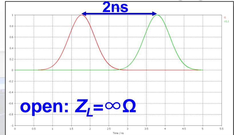
total reflection; reflected signal in phase, delay 2x1 ns.
