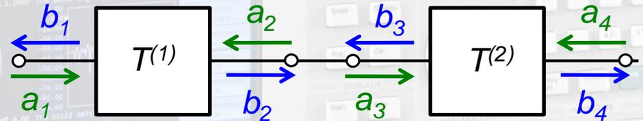
T-parameters can be directly evaluated from the associated S-parameters and vice versa.
