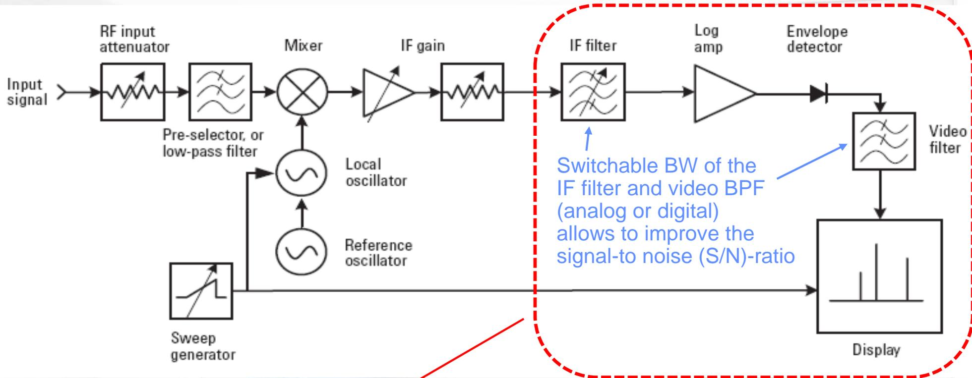
Today, the IF, demodulation, video and display sections of a spectrum analyzer are realized **digitally**
