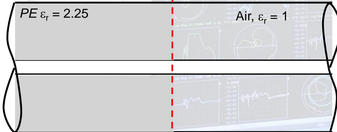
$t$  = voltage transmission coefficient, in this case:  $t = 1 + \Gamma$
