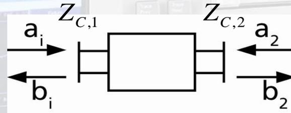
**Step 1:** Calculate the reflection coefficient and keep in mind: all ports have to be terminated with their respective characteristic impedance, i.e.  $75 \Omega$  for port 2.
