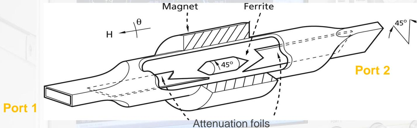
The left waveguide uses a  $TE_{10}$  mode (=vertically polarized H field). After transition to a circular waveguide, the polarization of the mode is rotated counter clockwise by  $45^\circ$  by a ferrite. Then follows a transition to another rectangular waveguide which is rotated by  $45^\circ$  such that the forward wave can pass unhindered. However, a wave coming from the other side will have its polarization rotated by  $45^\circ$  clockwise as seen from the right hand side.
