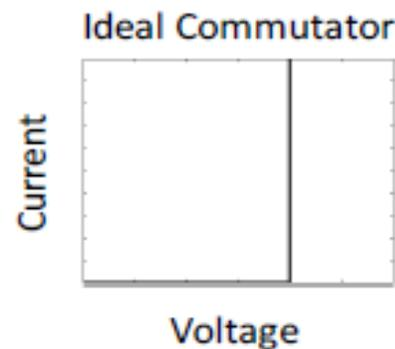
◆ The RF diode is NOT an ideal commutator for small signals! We cannot apply big signals otherwise burnout
