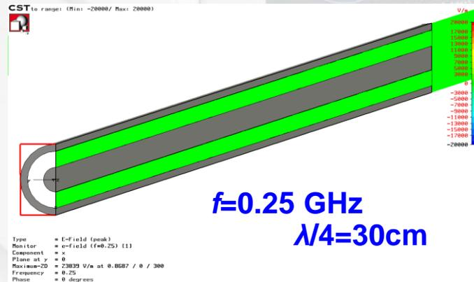
Coax cable with vacuum with a length of 30 cm
