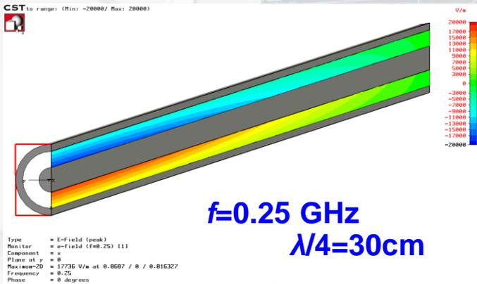
Coax cable with vacuum or air with a length of  $l=30$  cm
