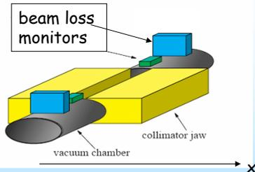
In a synchrotron one jaw will scrape both sides of the beam distribution ( $\beta$ -oscillation)
