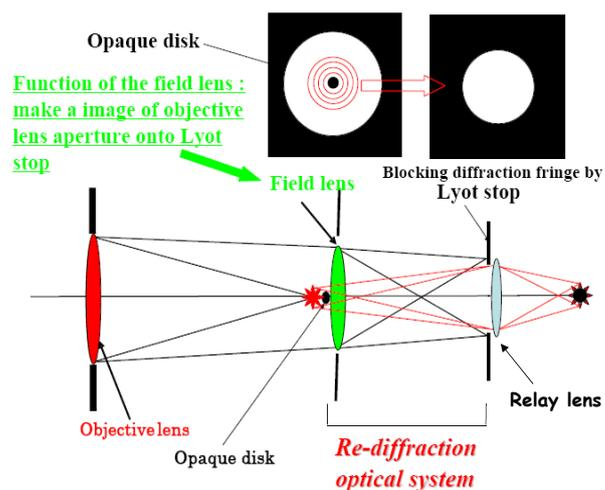
Then the re-diffracted light makes another diffraction fringe around the geometrical image of the objective lens aperture in the focal plane of the field lens. The Lyot stop removes this diffraction fringe by a mask, and relay the image by a third lens onto the final observation plane.
