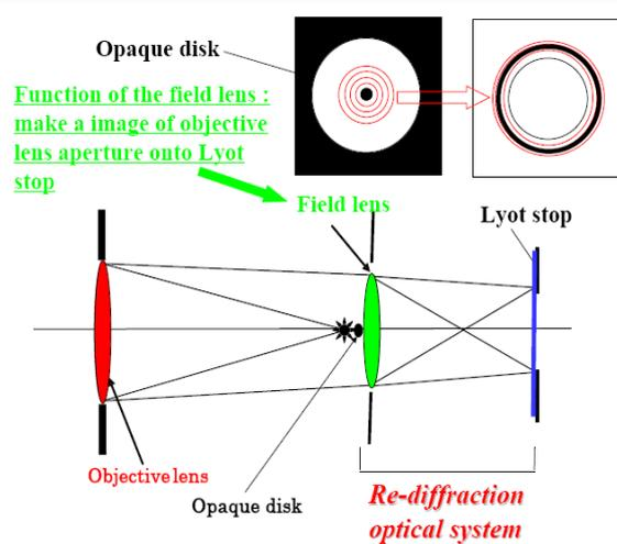
A second lens (field lens) is set just after the blocking disk. The focusing length of the field lens is chosen to make a real image of the objective lens aperture onto a mask (Lyot Stop).
