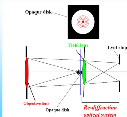
The first lens (objective lens) makes a real image of the object (beam image) on to a blocking opaque disk
