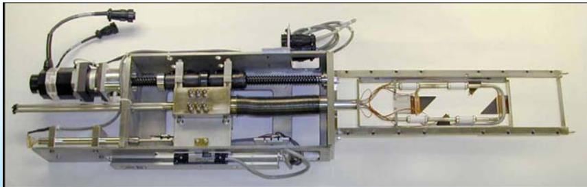
WS can move a 33- $\mu\text{m}$  carbon mono filament and two halo scraper consisting of two graphite scraping devices (one for each side of the distribution).
