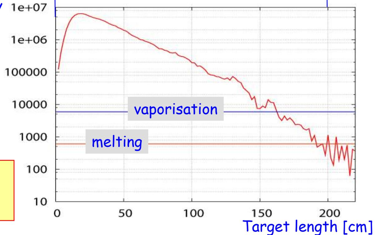
The beam will drill a hole along the target axis !!
