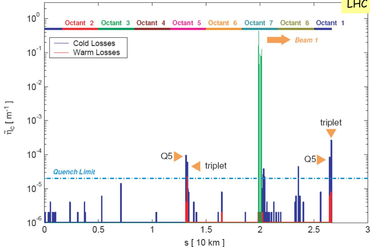
Impact distribution of protons scattered from the LHC collimator jaws at 7 TeV and tracked through the LHC lattice: indicates critical regions.
