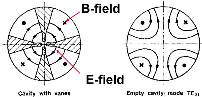
The  $TE_{210}$  mode in the “4-vane” structure and in the empty cavity.
