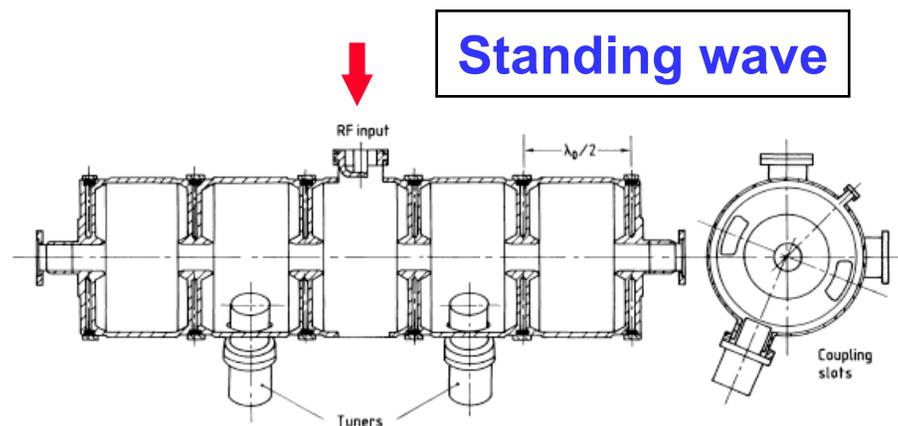
Chain of coupled cells in SW mode.
