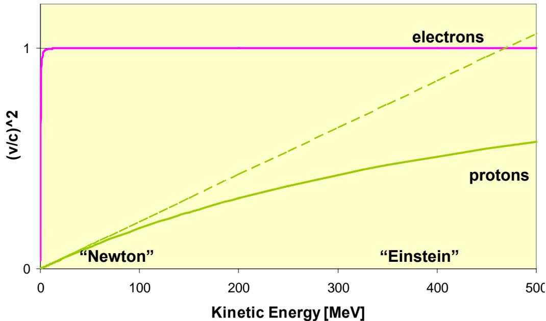
$\beta^2 = (v/c)^2$  as function of kinetic energy  $T$  for protons and electrons.
