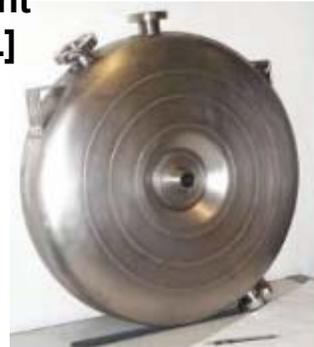
Superconducting linacs for low and medium beta ions are made of multi-gap (1 to 4) individual cavities, spaced by focusing elements. Advantages: can be individually phased → linac can accept different ions
