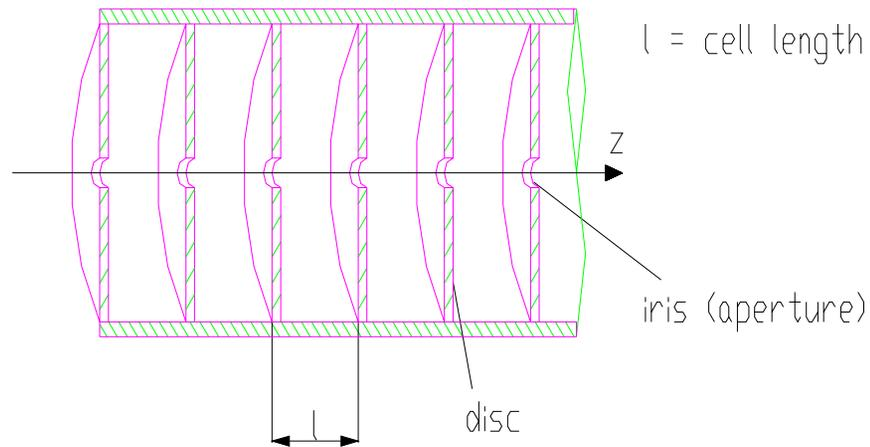
Discs inside the cylindrical waveguide, spaced by a distance  $\ell$ , will induce multiple reflections between the discs.
