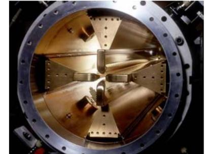
Alternative resonator design: the “4-rod” structure, where an array of  $\lambda/4$  parallel plate lines loads four rods, connected in such a way as to provide the quadrupole field.
