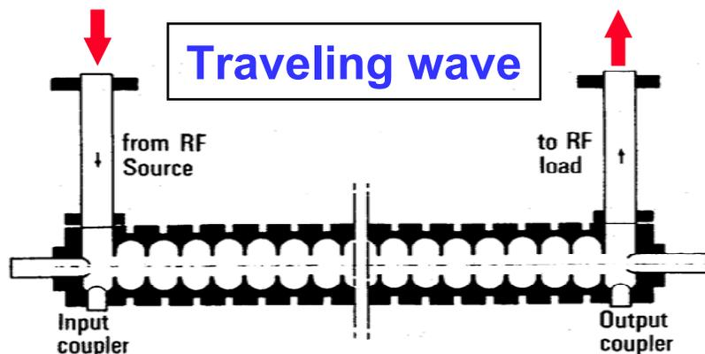
Chain of coupled cells in TW mode
