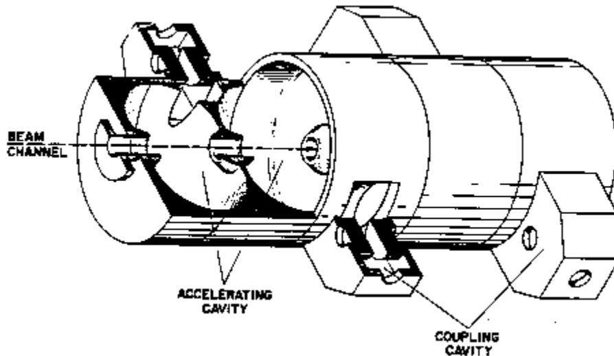
Example: the Cell-Coupled Linac at SNS, >100 cells/module
