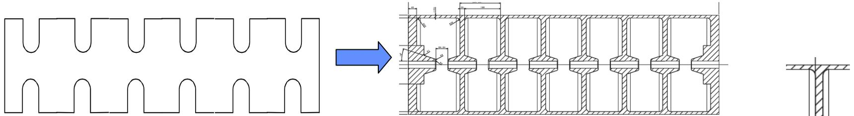
From **disc-loaded structure** to a **real cavity** (Linac4 PIMS, Pi-Mode Structure)
