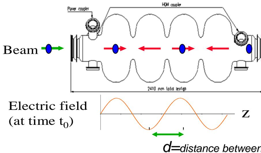
Example: a linac superconducting 4-cell accelerating structure
