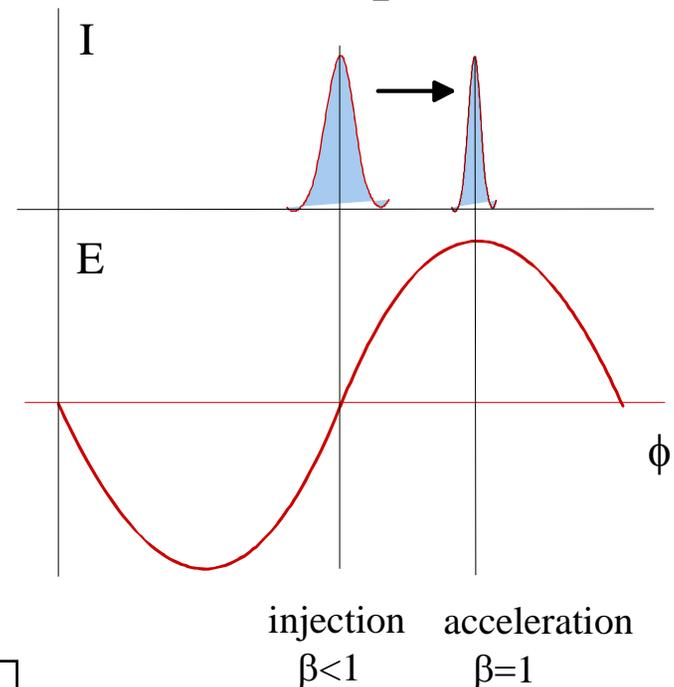
In high current linacs, a bunching and pre-acceleration sections up to 4-10 MeV prepares the injection in the TW structure (that occurs already on the crest)
