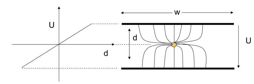
If the beam is much smaller than w, all field lines are captured and U is a linear function with replacement else: Linear cut (projection to measurement plane must be linear)
