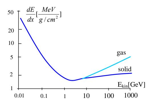
Heavy ions at low energy are stopped within a few micro-meters All energy is deposited in a very small volume
