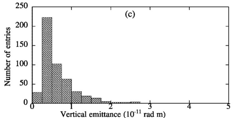
Simulations of emittance tuning in the ATF damping ring.
