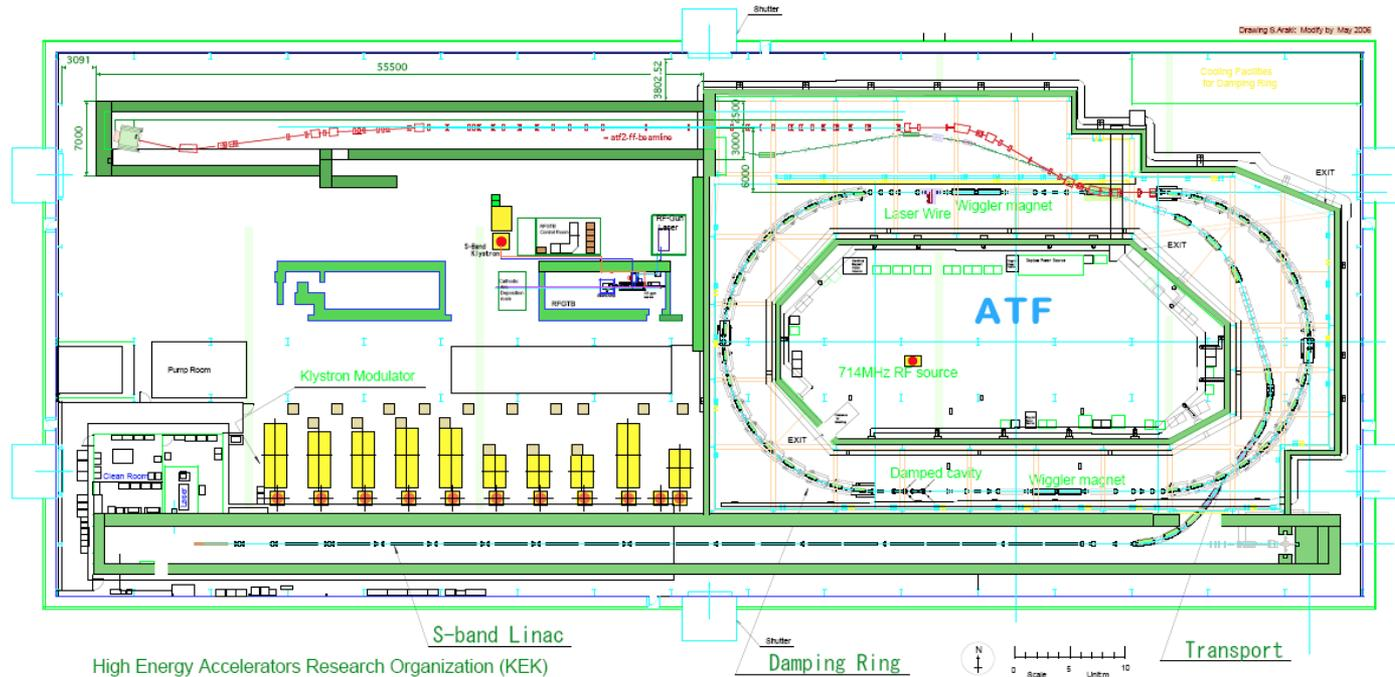
The main components are a 1.28 GeV S-band linac, a 1.28 GeV storage ring, and an extraction line. The extraction line is presently being extended (ATF2) to provide a test facility for linear collider beam delivery systems.
