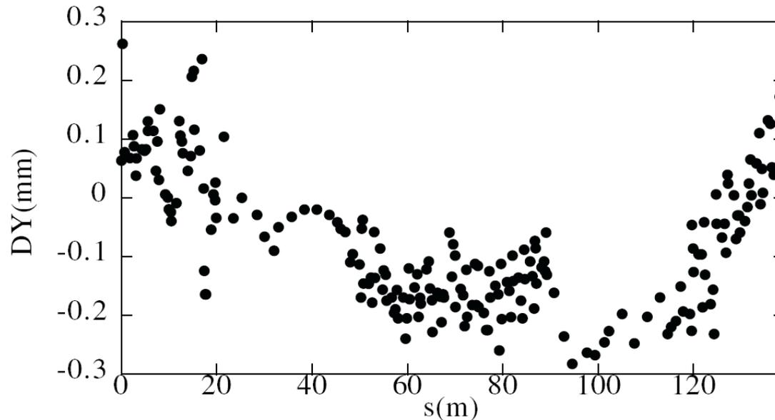
Vertical alignment of the magnets is critical:
