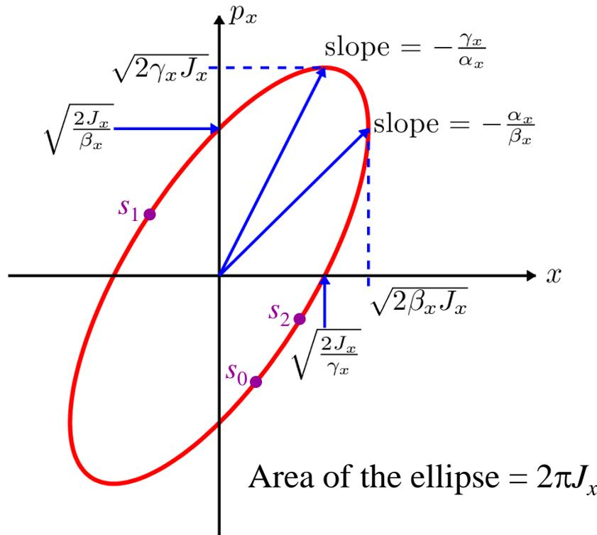
In an *uncoupled* periodic beam line, particles trace out ellipses in phase space with each pass through the periodic cell. The shape of the ellipse defines the *Twiss parameters* at the observation point.
