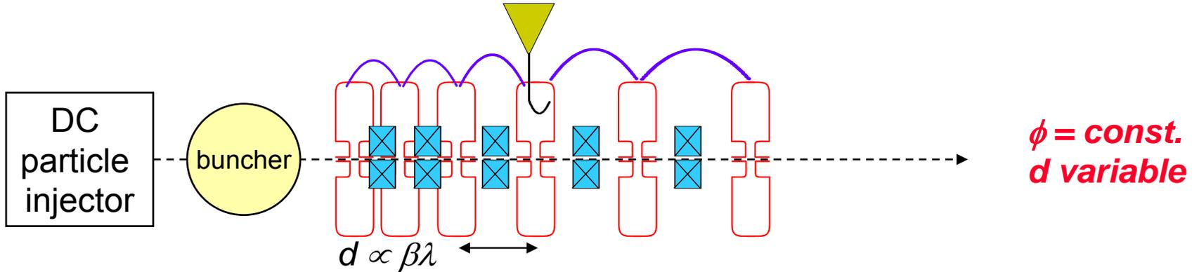
$\Phi$  = phase difference between 2 adjacent accelerating cells, defined by the type of coupling
