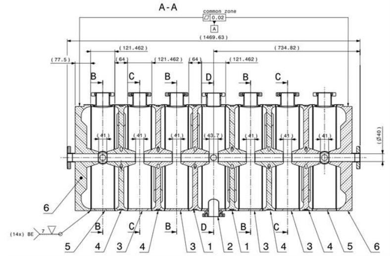
This structure is composed of 7 accelerating cells, magnetically coupled.
