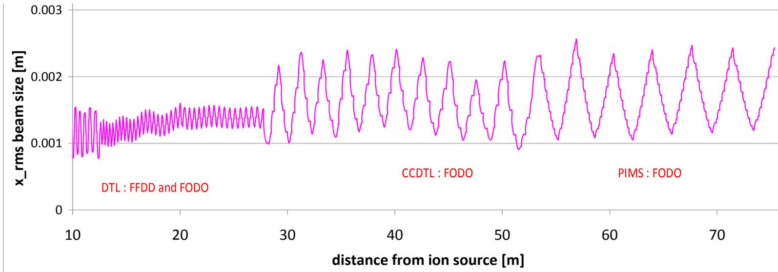
Example: beam dynamics design for Linac4@CERN.
