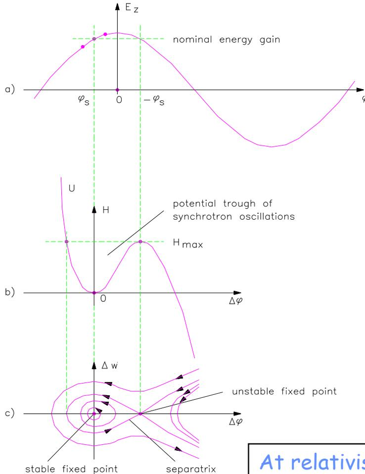
→ Ions are accelerated around a (negative = linac definition) synchronous phase.
