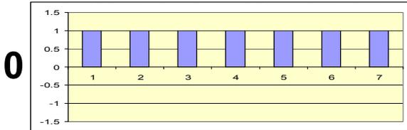
$$\Phi = 2\pi, \quad 2\pi \frac{d}{\beta\lambda} = 2\pi, \quad d = \beta\lambda$$
