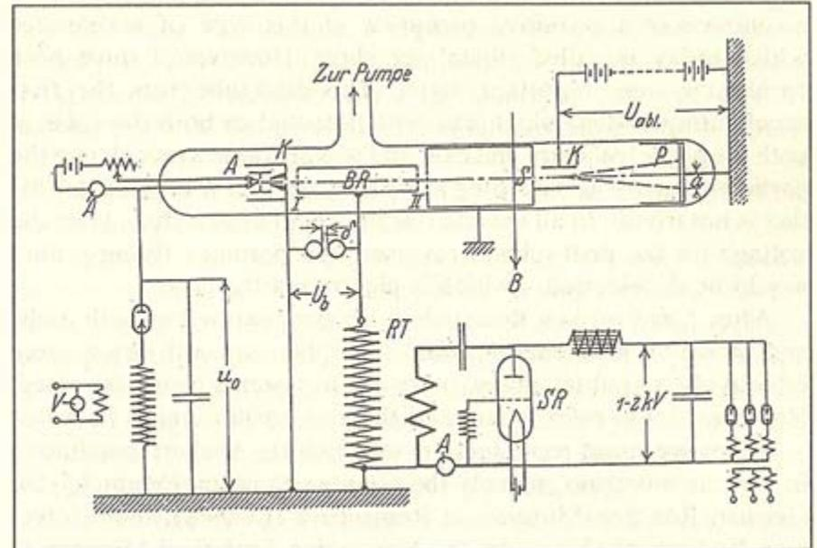
Fig. 3.6: Acceleration tube and switching circuits [Wi28].
