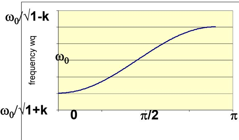
All modes in the dispersion curve are allowed, the original frequency degenerates into a continuous band. The field is the same in each cell, there are no more standing wave modes → only “traveling wave modes”, if we excite the EM field at one end of the structure it will propagate towards the other end.
