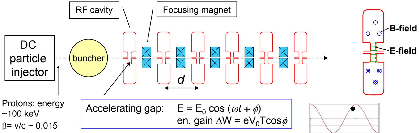
Acceleration  $\rightarrow$  the beam has to pass in each cavity on a phase  $\phi$  near the crest of the wave
