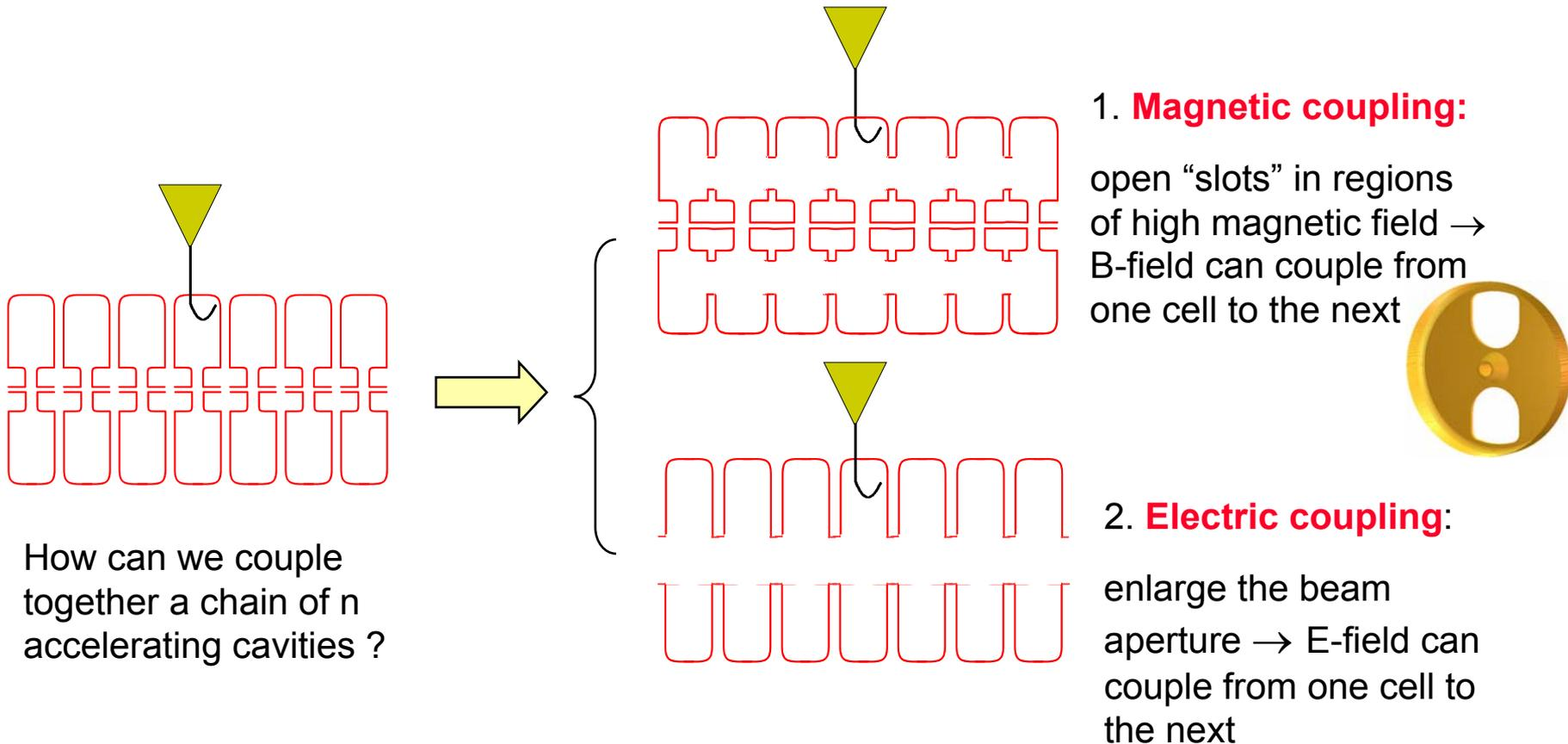
The effect of the coupling is that the cells no longer resonate independently, but will have common resonances with well defined field patterns.
