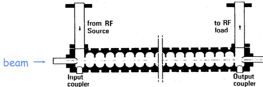
“Disc-loaded waveguide” or chain of electrically coupled cells characterized by a continuous band of frequencies. In the chain is excited a “traveling wave mode” that has a propagation velocity  $v_{ph} = \omega/k$  given by the dispersion relation.
