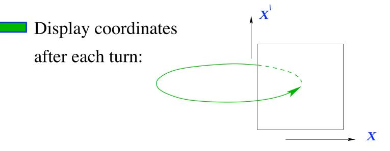
the ellipse orientation and the half axis length vary along the machine
