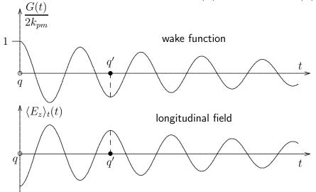
G(t) is related to longitudinal field  $E_z$  by an integration following the particle with  $v \approx c$  and taking momentary field value
