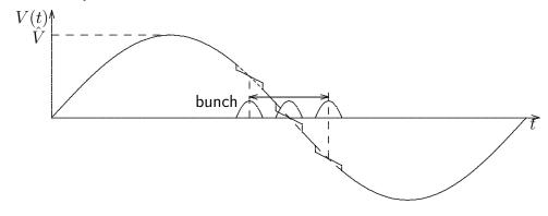
Reduction of  $\omega_s$  reduces longitudinal focusing and increases the bunch length
