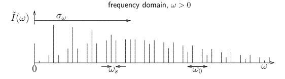
Bunch executing synchrotron oscillation with  $\omega_s = \omega_0 Q_s$  and amplitude  $\hat{\tau}$  modulates passage time  $t_k$  at cavity in successive turns k
