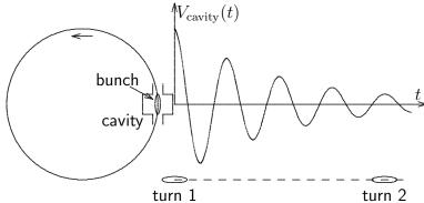
Single traversal effects driven by strong self-fields from broad impedances change distribution, modify oscillation modes and can couple them. Self consistent solutions are difficult to get, bunch lengthening.
