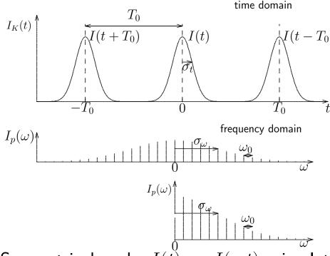
Symmetric bunch, I(t)=I(-t), circulates with turns k of duration  $T_0$ , is a periodic current and expressed by a Fourier series
