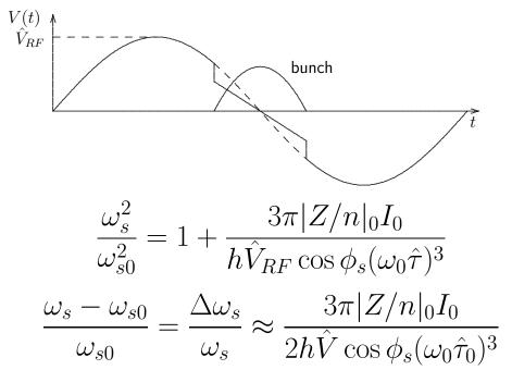
Only incoherent frequency of single particles is changed (reduced for  $\gamma > \gamma_T$ , increased for  $\gamma < \gamma_T$ ), but not the coherent dipole (rigid bunch) mode. This separates the two.
