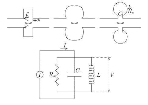
Cavities have narrow band oscillation modes which can drive coupled bunch instabilities. Each resembles an **RCL** - **circuit** and can, in good approximation, be treated as such. This circuit has a shunt impedance  $R_s$ , an inductance L and a capacity C. In a real cavity these parameters cannot easily be separated and we use others which can be measured directly: The **resonance frequency**  $\omega_r$ , the **quality factor** Q and the **damping rate**  $\alpha$ :
