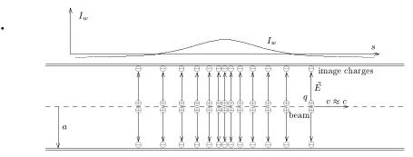
Beam induces wall current  $I_w = -(I_b - \langle I_b \rangle)$
