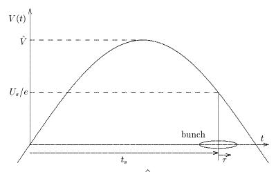
RF-cavity of voltage  $\hat{V}$ , frequency  $\omega_{\rm RF}=h\omega_0$ , SR energy loss U the energy gain or loss of a particle in one turn  $\delta\epsilon=\delta E/E$  is
