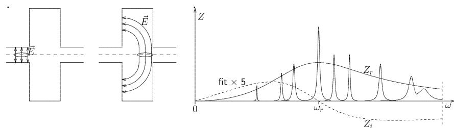
Aperture changes form cavity-like objects with  $\omega_r$ ,  $R_s$  and Q and impedance  $Z(\omega)$  developed for  $\omega < \omega_r$ , where it is inductive
