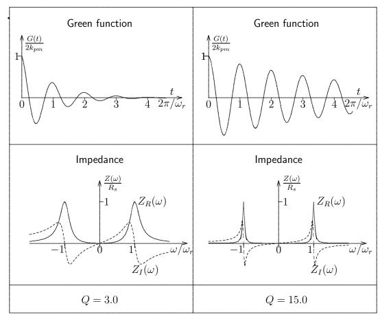
$$Z(\omega) = R_s \frac{1 - jQ \frac{\omega^2 - \omega_r^2}{\omega \omega_r}}{1 + Q^2 \left(\frac{\omega^2 - \omega_r^2}{\omega \omega_r}\right)^2} = Z_r + jZ_i$$
