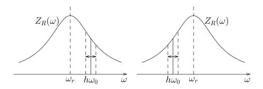
Important longitudinal instability of a bunch interacting with an narrow impedance, called **Robinson** instability. In a qualitative approach we take single bunch and a narrow-band cavity of resonance frequency  $\omega_r$  and impedance  $Z(\omega)$  taking only its resistive part  $Z_r$ . The revolution frequency  $\omega_0$  depends on energy deviation  $\Delta E$
