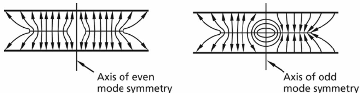
Fig. 21: Even and odd mode in coupled striplines [14]
