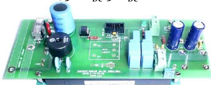
600 W, 300 V DC /30 V DC converter
