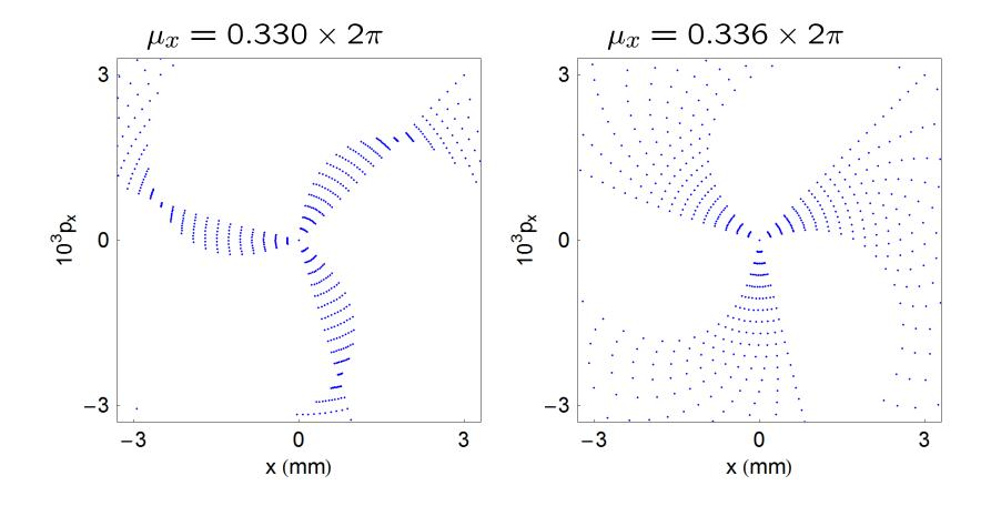
"Islands" appear in phase space portraits at amplitudes where the phase advance is  $2\pi \times$  a rational number (that determines the number of islands), and where the transfer map contains a "driving term" (that determines the widths of the islands).
