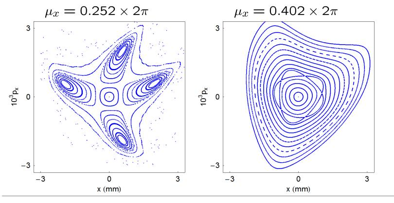
Perturbation theory and normal form analysis depend on the existence of constants of motion in the presence of nonlinear perturbations.
