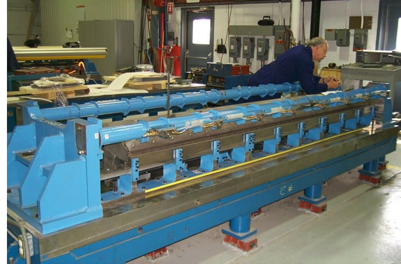
Stacking an MQW quadrupole yoke stack
