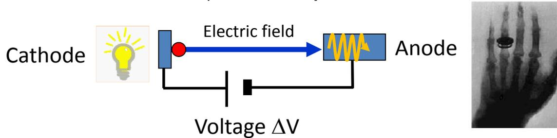
The **energy gained** by the electrons travelling from the cathode to the anode is equal to their charge multiplied the DC voltage between the two electrodes.
