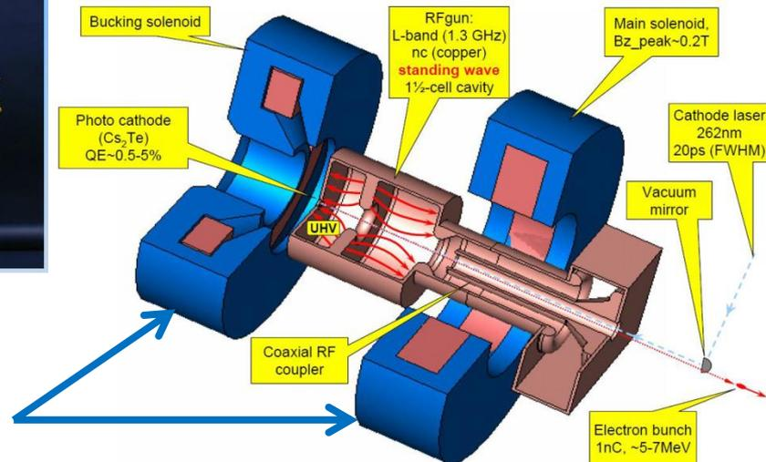
Solenoids field are used to compensate the space charge effects in low energy guns. The configuration is shown in the picture
