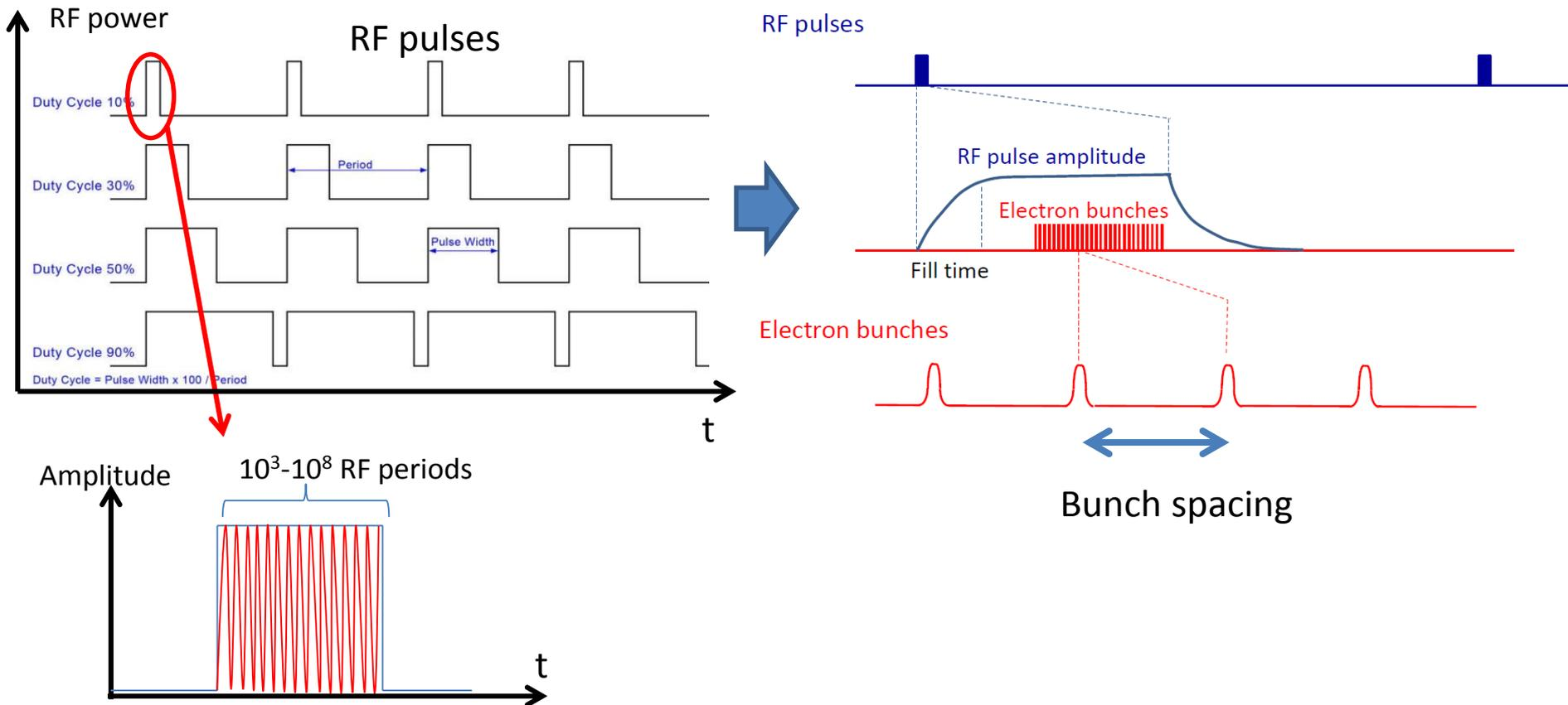
$\Rightarrow$  Because of the very low power dissipation and low RF power required to achieve a certain accelerating voltage the **SC structures allow operation at very high Duty Cycle (DC) up to a CW operation with high gradient (>20 MV/m)**.
