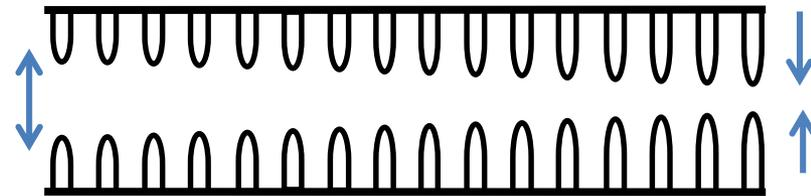
In a purely periodic structure, made by a sequence of **identical cells** (also called “**constant impedance structure**”), the RF power flux and the intensity of the accelerating field decay exponentially along the structure :
