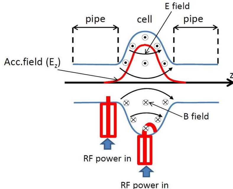
For a **pure cylindrical structure** (also called **pillbox cavity**) the first accelerating mode (i.e. with non zero longitudinal electric field on axis) is the **TM<sub>010</sub> mode**. It has a well known analytical solution from Maxwell equation.
