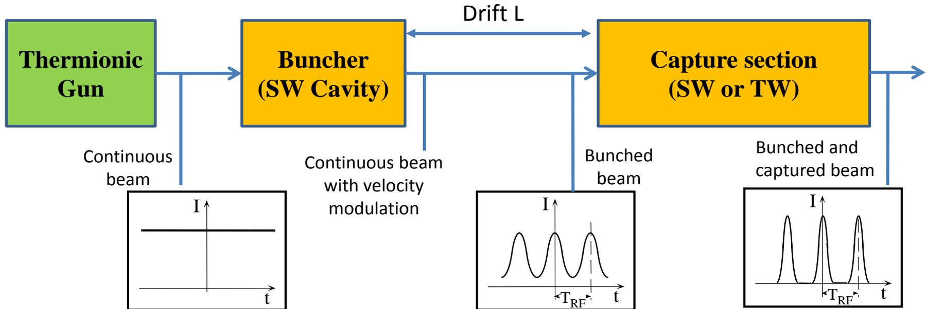
⇒ **Bunching** is obtained by modulating the energy (and therefore the velocity) of a continuous beam using the longitudinal E-field of a SW cavity. After a certain **drift space** the **velocity modulation is converted in a density charge modulation**. The density modulation depletes the regions corresponding to injection phase values incompatible with the capture process
