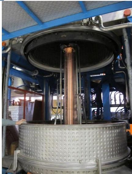
The cells are then piled up and **brazed** together in vacuum or hydrogen furnace using different alloys at different temperatures (700-1000 C) and/or in different steps.
