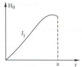
$$E_z = AJ_0\left(2.405\frac{r}{a}\right)\cos(\omega_{RF}t) \quad H_\theta = A\frac{1}{Z_0}J_1\left(2.405\frac{r}{a}\right)\sin(\omega_{RF}t)$$
