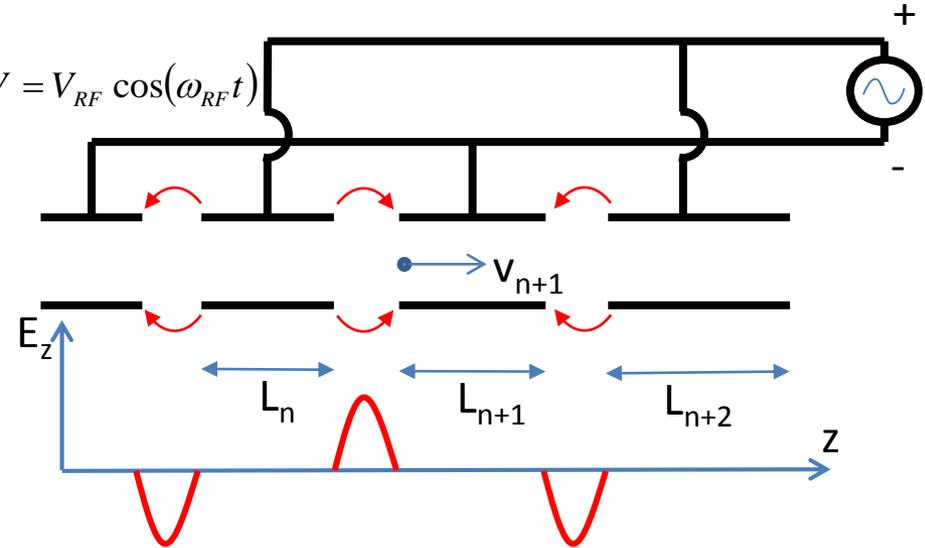
⇒ In order to be synchronous with the accelerating field at each gap the **length of the n-th drift tube** has to be  $L_n$ :
