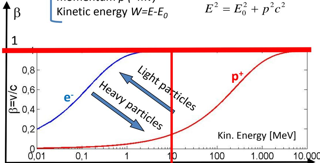
⇒ **Light particles** (as **electrons**) are practically fully relativistic ( $\beta \approx 1$ ,  $\gamma \gg 1$ ) at relatively low energy and **reach a constant velocity** ( $\sim c$ ). The acceleration process occurs at constant particle velocity
