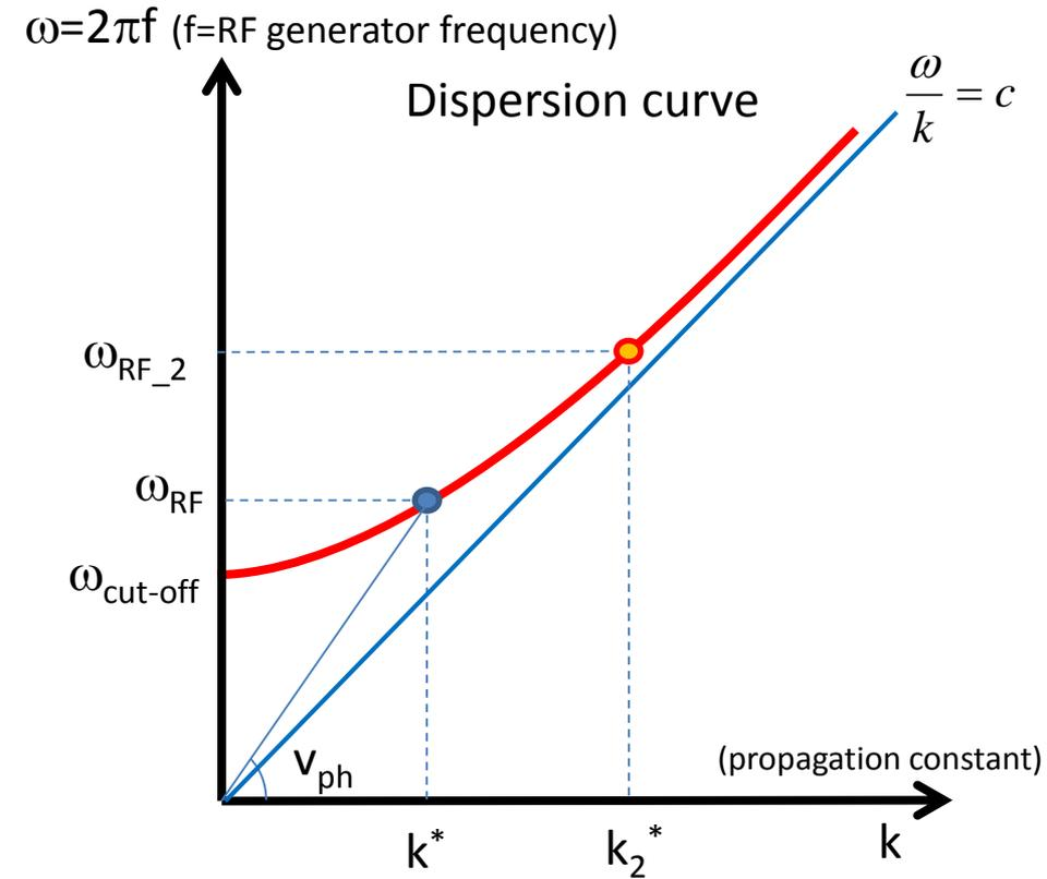
As example if we consider a simple circular waveguide the first propagating mode with  $E_z \neq 0$  is the  $TM_{01}$  mode. Nevertheless by solving the wave equation it turns out that an e.m. wave propagating in this **constant cross section waveguide** will **never be synchronous with a particle beam** since the **phase velocity is always larger than the speed of light  $c$** .
