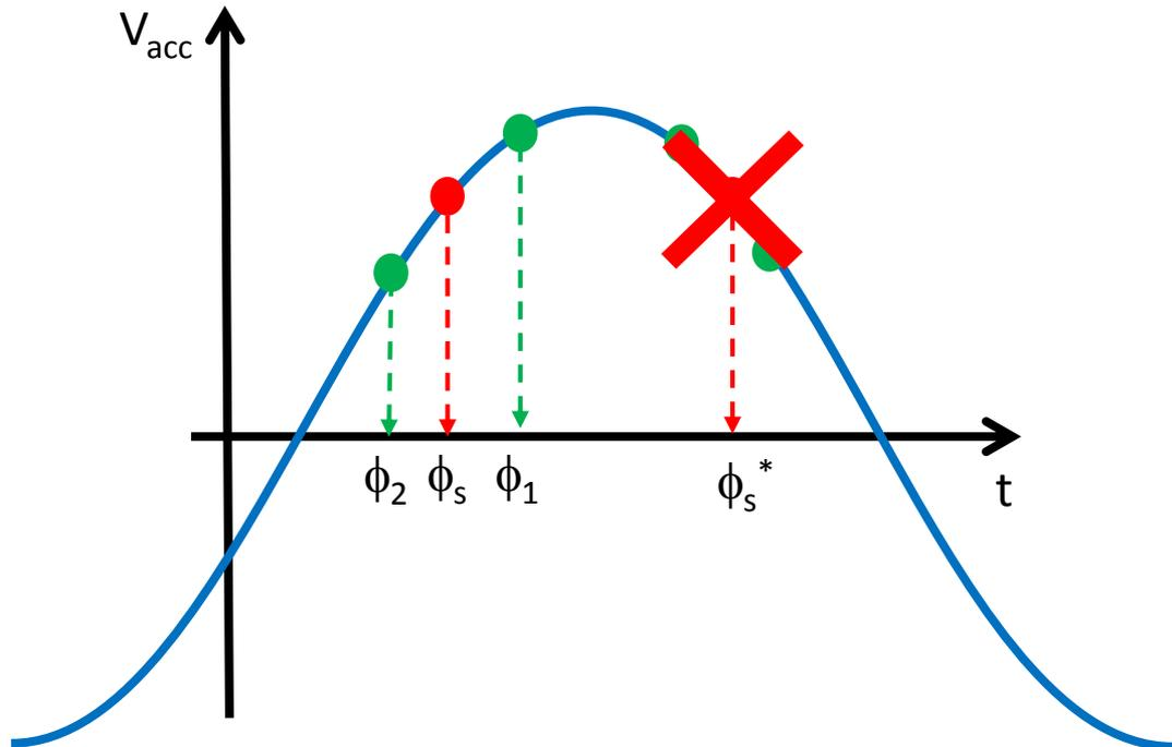
⇒ The choice of the synchronous phase in the positive slope of the RF voltage provides longitudinal focusing of the beam: **phase stability principle**.
