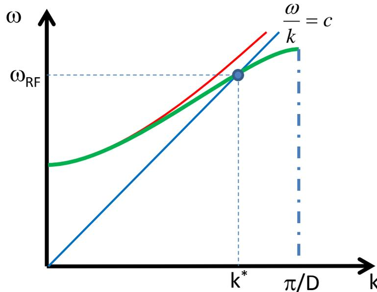
⇒ The structure can be designed to have the **phase velocity equal to the speed of the particles**.
