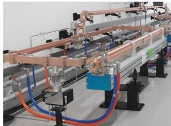
Focusing elements: quadrupoles and solenoids
