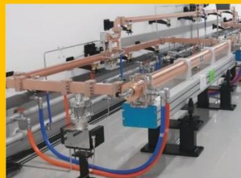
Focusing elements: quadrupoles and solenoids
