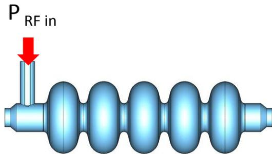
Is equivalent to the **superposition of two counterpropagating TW waves**
