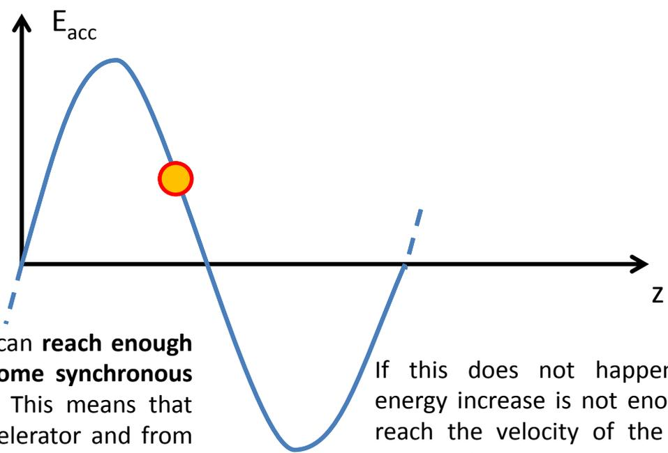
After a certain distance they can **reach enough energy (and velocity) to become synchronous** with the accelerating wave. This means that they are captured by the accelerator and from this point they are stably accelerated.
