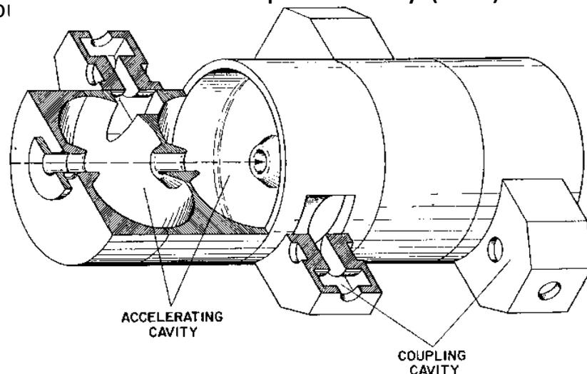
$f_{RF} = 800 - 3000$  MHz for proton ( $\beta = 0.5-1$ ) and electrons
