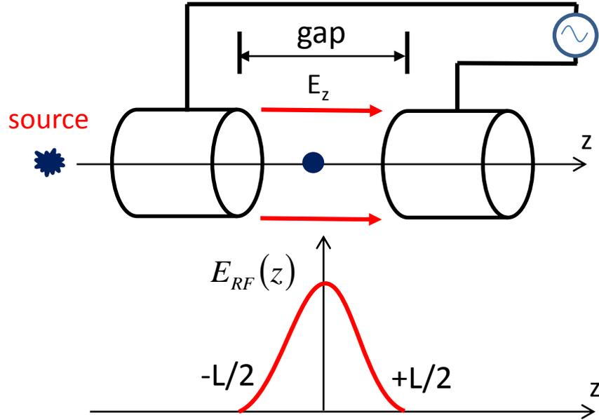
$$\Delta V = V_{RF} \cos(\omega_{RF} t) \quad \omega_{RF} = 2\pi f_{RF} = \frac{2\pi}{T_{RF}}$$
