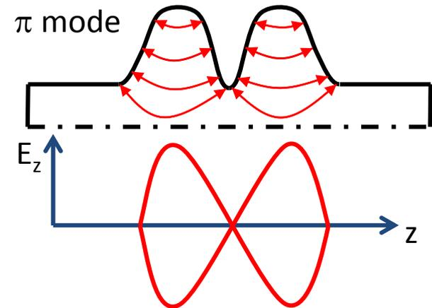
⇒ For **ions and protons** the cell length has to be increased and the linac will be made of a sequence of different accelerating structures matched to the ion/proton velocity.
