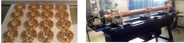
The most widely used NC metal for RF structures is **OFHC copper** (Oxygen free high conductivity) for several reasons:
