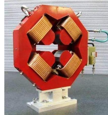
Electromagnetic quadrupoles  $G < 50\text{-}100 \text{ T/m}$
