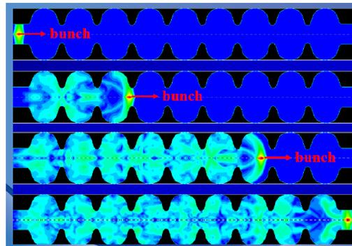
Several approaches are used to absorb these field from the structures like **loops** couplers, **waveguides**, Beam pipe **absorbers**
