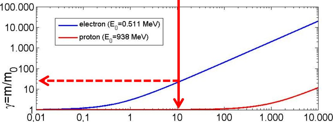
⇒ This implies **important differences** in the technical characteristics of the **accelerating structures**. In particular for **protons and ions** we need different types of accelerating structures, **optimized for different velocities** and/or the accelerating structure has to vary its geometry to take into account the velocity variation.
