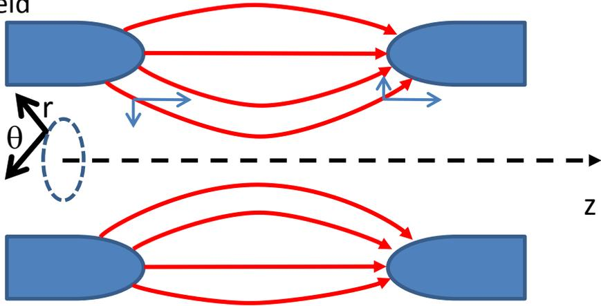
⇒ According to Maxwell equations the **divergence of the field is zero** and this implies that in traversing one accelerating gap there is a focusing/defocusing term
