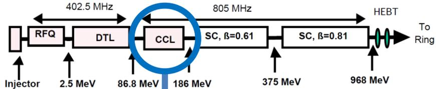
4 modules, each containing 12 accelerator segments CCL and 11 bridge couplers. The CCL section is a RF Linac, operating at **805 MHz** that accelerates the beam **from 87 to 186 MeV** and has a physical installed length of slightly over **55 meters**.
