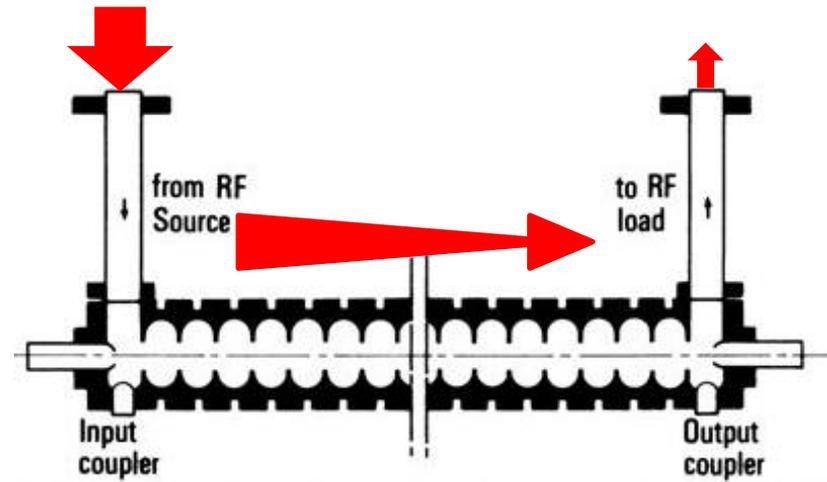
It is possible to demonstrate that, in order to keep the **accelerating field constant** along the structure, the **iris apertures have to decrease along the structure**.
