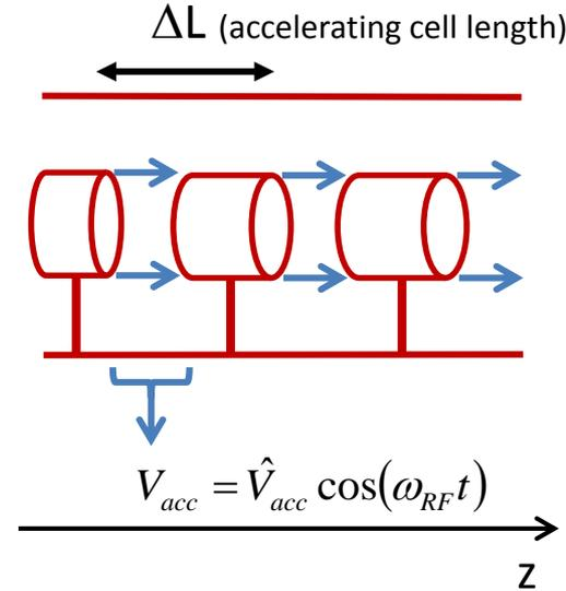
The **energy gain per cell (one gap + tube in case of a DTL)** of a generic particle and of a synchronous particle are (we put  $\theta=0$  in the generic expression of the accelerating voltage just for simplicity):
