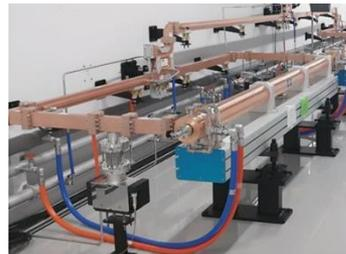
Focusing elements: quadrupoles and solenoids
