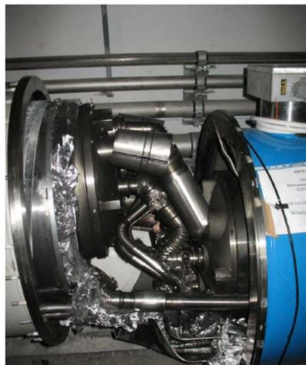
Accidental release of an energy of 600 MJoule stored in the magnet system - No Beam
