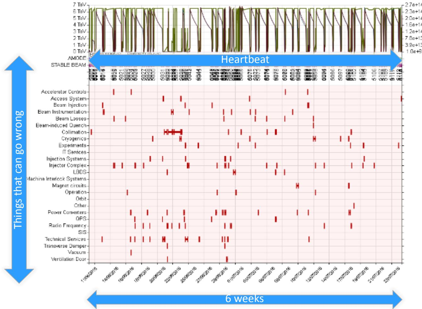
Introduced in Run2 a common metrics and tracking of LHC downtime and root causes
