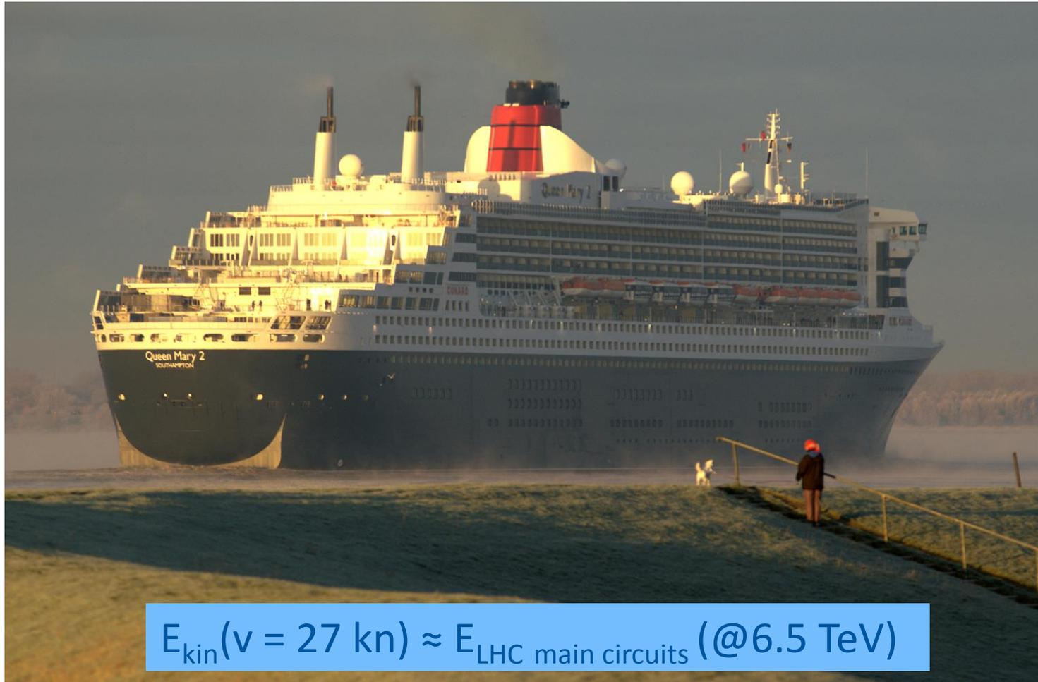
$$E_{\text{kin}}(v = 27 \text{ kn}) \approx E_{\text{LHC main circuits}} (@6.5 \text{ TeV})$$
