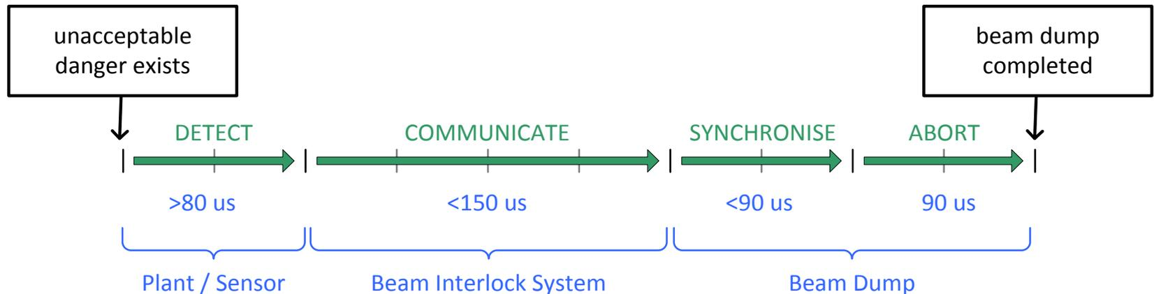
At the LHC the delay can be as much as  $\sim 3$  turns –  $\sim 300$  us
