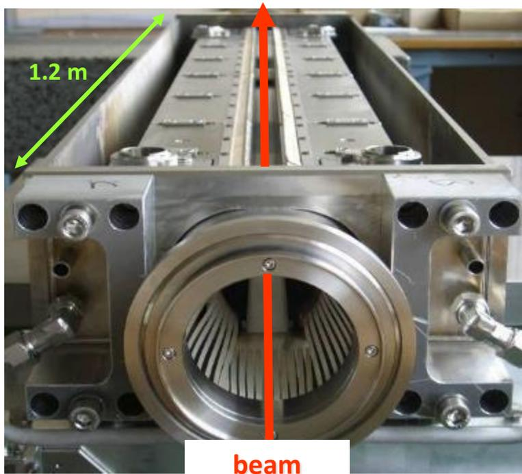
Almost **100 collimators**, mostly made of Carbon and Tungsten, protect the superconducting magnets against energy deposition from the beam
