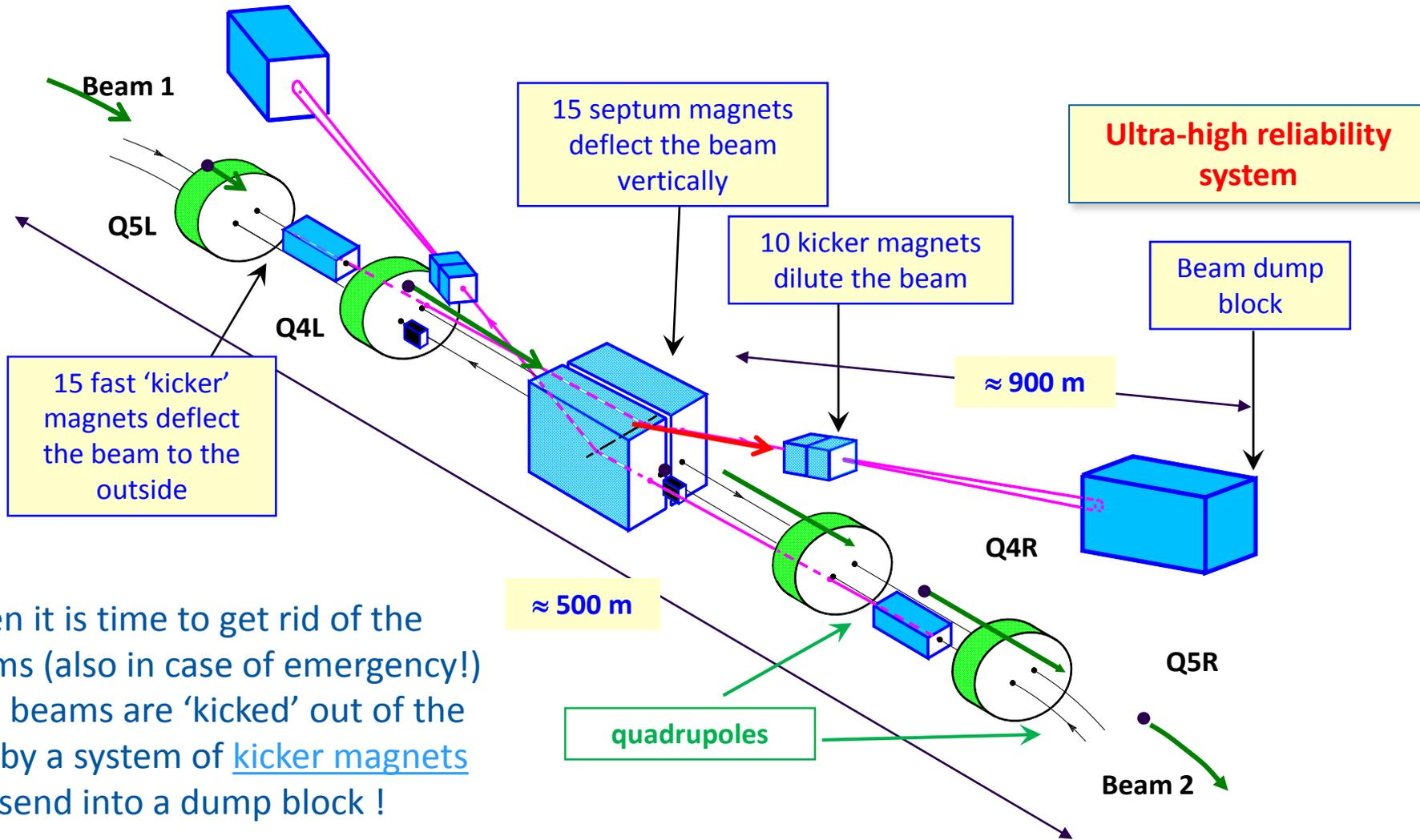
When it is time to get rid of the beams (also in case of emergency!), the beams are 'kicked' out of the ring by a system of kicker magnets and send into a dump block !
