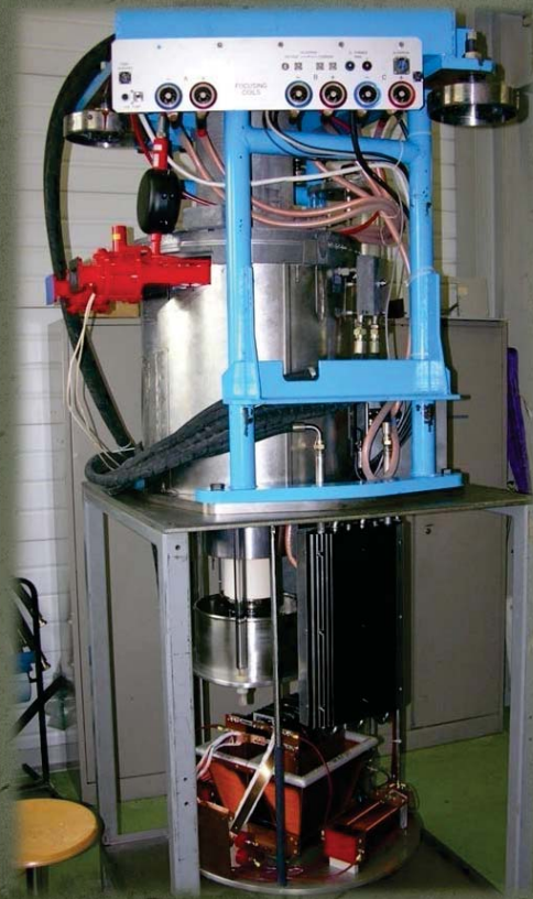
CERN CTF3 (LIL): 3 GHz, 45 MW, 4.5 \mu s, 50 Hz, \eta 45 %
