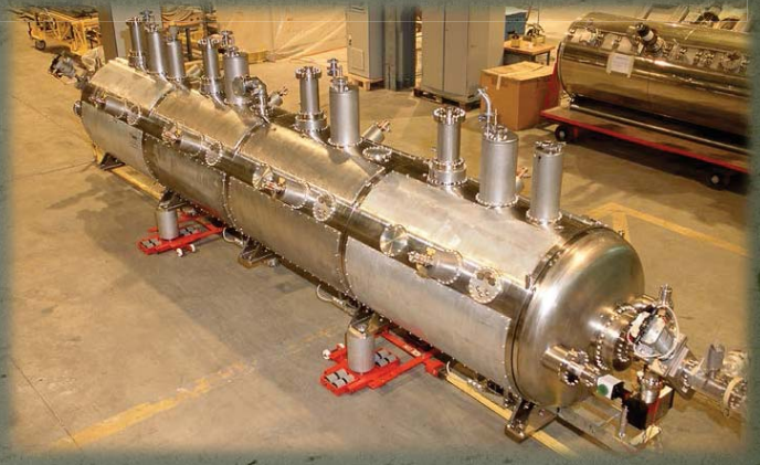
LHC spare module stored in CERN's SM18
