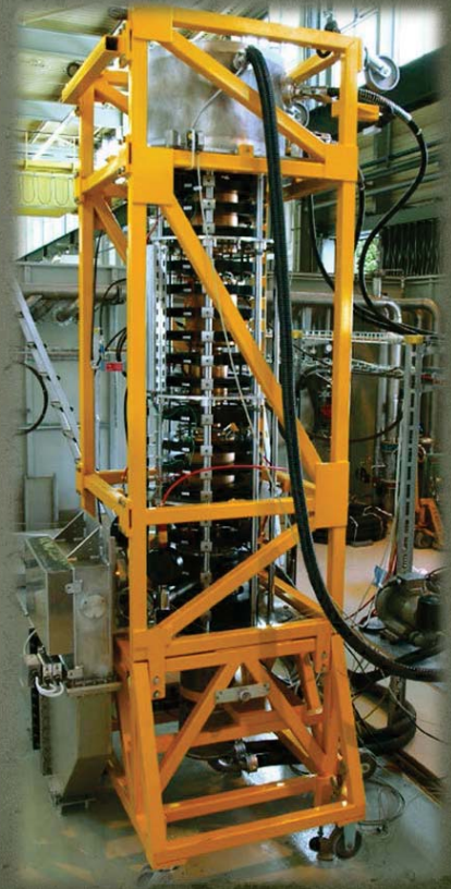
CERN LHC: 400 MHz, 300 kW, CW, \eta 62 %
