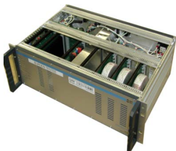
13kA DCCT Electronics
