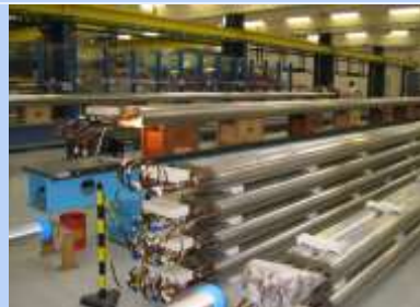
Collared coils ready for cold mass assembly
