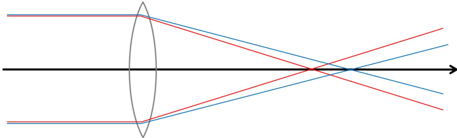
The change in focusing strength with particle energy has undesirable consequences, especially in storage rings: it can lead to particle motion becoming unstable because of resonances.
