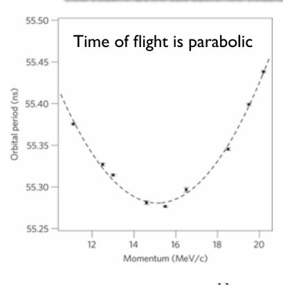
Suppose we choose rf frequency that is synchronized with revolution frequency at the center.
