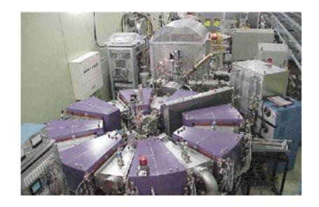
Proof of Principle machine finished in 1999 at KEK, demonstrated 1kHz rep. rate
