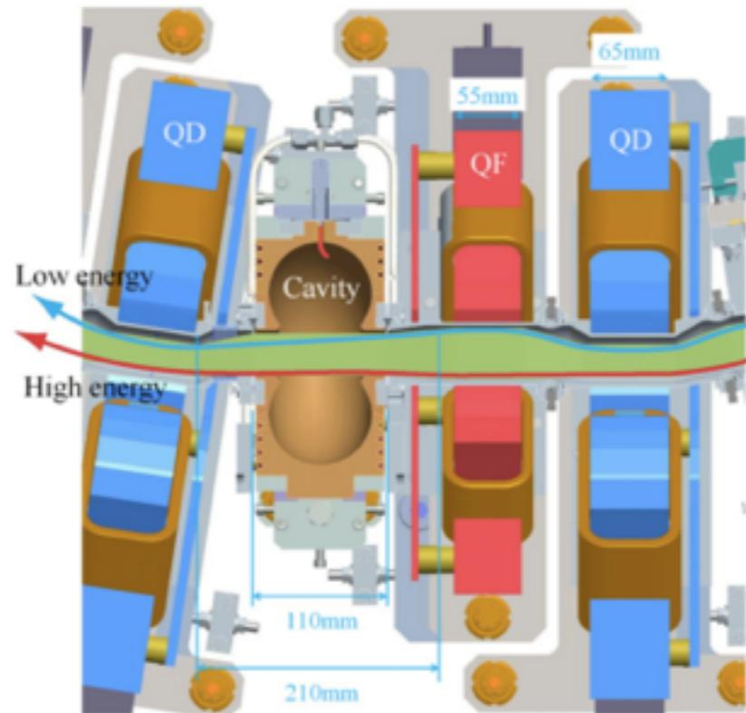
Quadrupole with radial offset creates bending component
