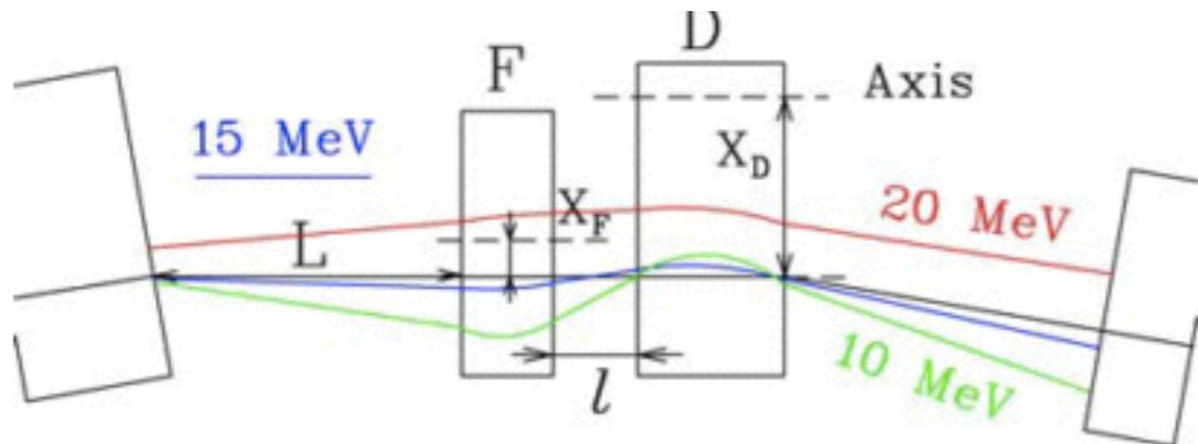
If the total time lag is less than a half of rf cycle, a beam has net energy gain.
