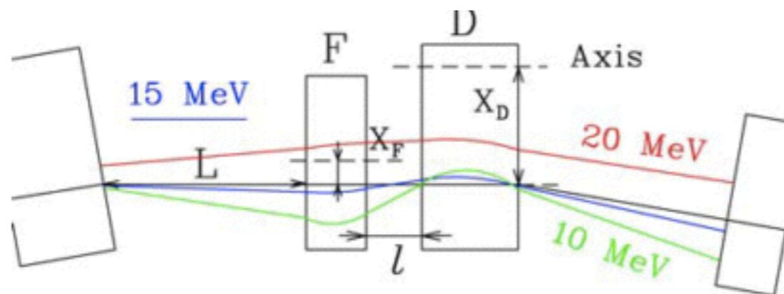
Figure 2: Orbits in a quadrupole doublet cell.
