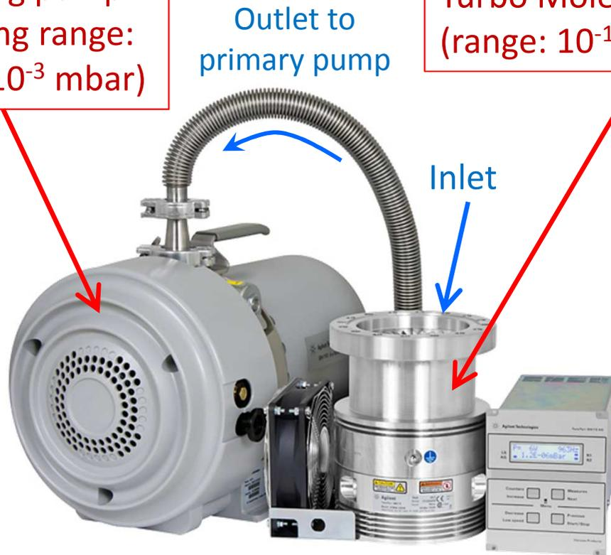
Turbo molecular and roughing pump connected in series:
