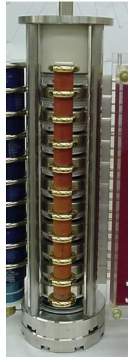
Stack of high-power semiconductor switches (GTOs)
