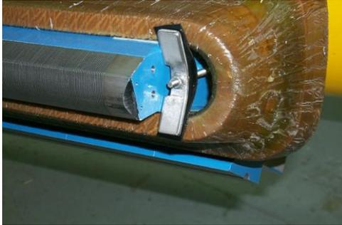
coil electrical test (under water !)
