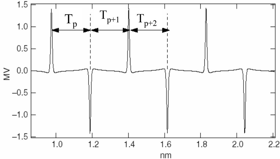
Horizontal electric field produced on-axis by a single 6 GeV electron propagating through an undulator with a 34 mm period and a 0.7 T peak field.
