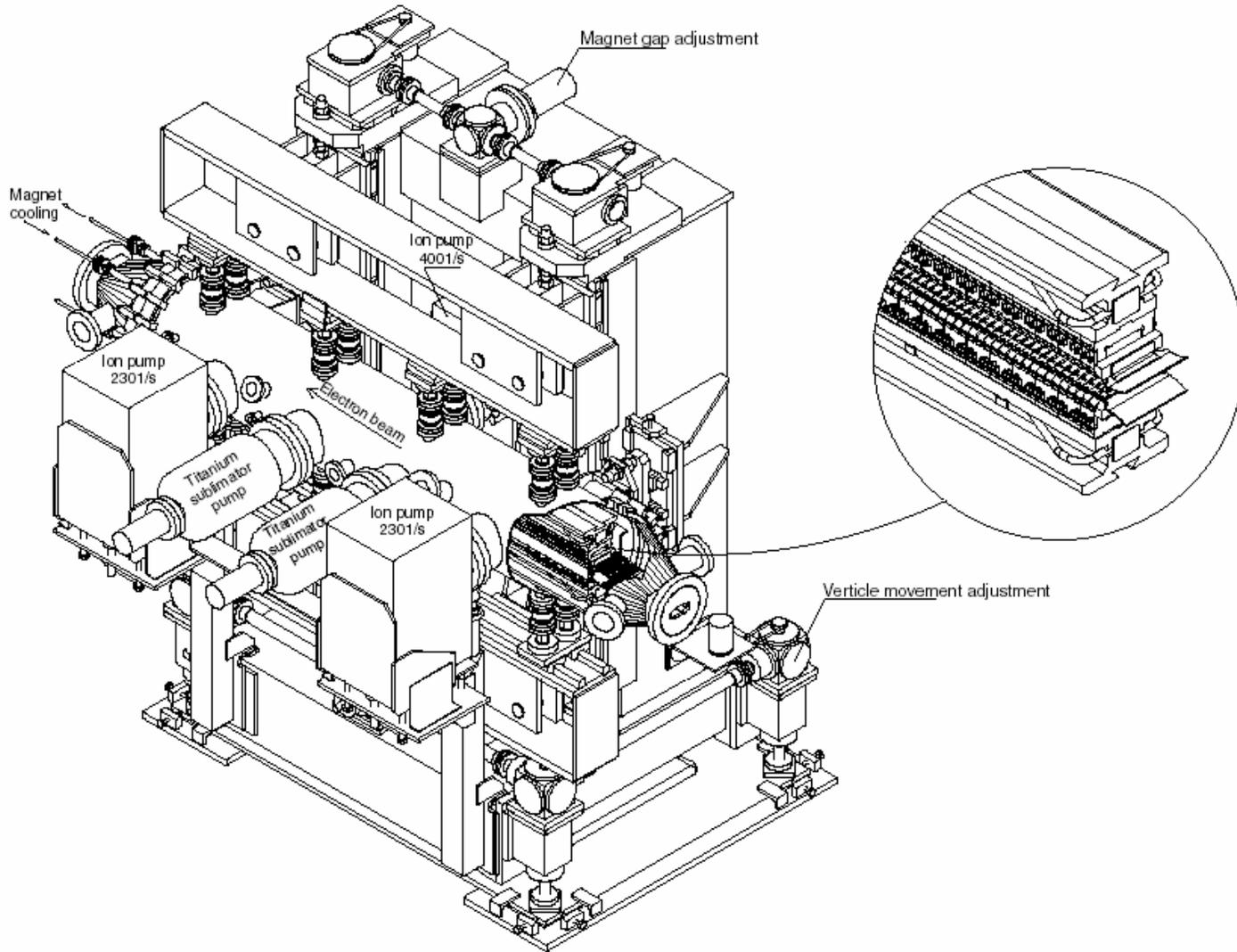
Figure 5.26 3D view of an ESRF in-vacuum undulator.
