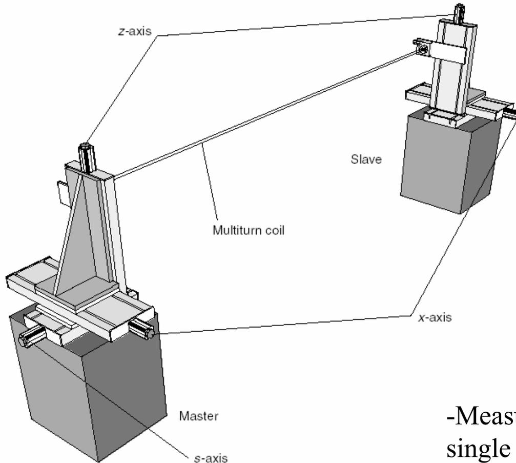
Figure 5.16 View of a field integral measuring bench.
