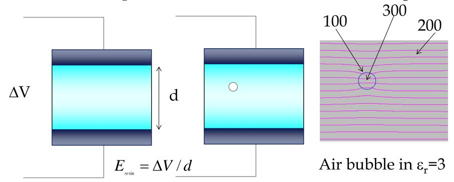
As  $\varepsilon_{resin} > \varepsilon_{air}$  the electric field in an air bubble can be much higher than the average one in the dielectric medium ! Also, as in general air is less insulating than a good dielectric, easily electrical discharges can appear in the bubble (see later).
