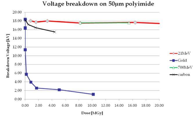
Ion beam induced degradation of polyimide is not only depending on the absorbed dose : the ion type plays a major role. The analysis of pre-discharge current patterns suggests different forms of damage depending on the irradiation type. Investigations of these effects on polyimide and on other materials are under way.
