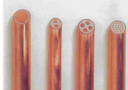
Used in Fire Protection, Nuclear Plants, Thermocouples, Magnets Hygroscopic, shall be sealed in the ends Not suitable for voltages > 1000 V
