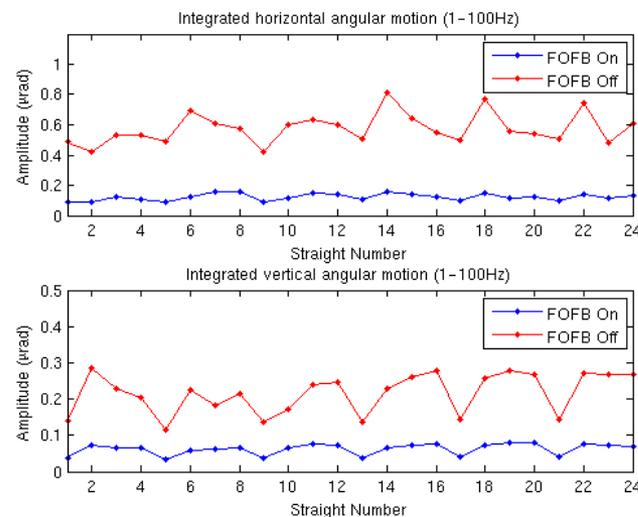
Integrated motion in the 1-100Hz bandwidth in each straight section of Diamond with FOFB on and off.
