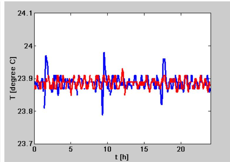
Left: ALS LCW temperature, Right: Tunnel air temperature (red – with top-off)
