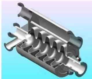
Standing wave structures for particles at  $\beta > 0.5-0.7$ , widely used for protons (SNS, etc.) and electrons (ILC, etc.)
