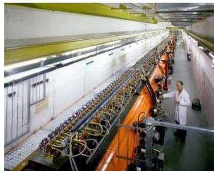
Top; CERN Linac2 Drift Tube Linac accelerating tank 1 (200 MHz). The tank is 7m long (diameter 1m) and provides an energy gain of 10 MeV.
