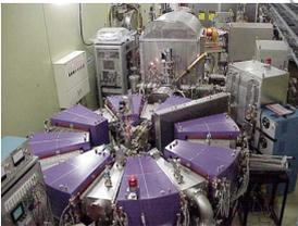
Nonscaling FFAG uses simple shifted Quad (to produce Bend field.)
