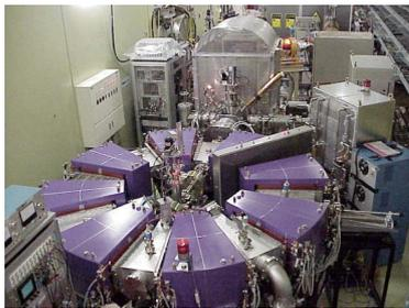
Proof of principle (proton acceleration with rf cavity) machine was constructed in 1999 and demonstrate rapid acceleration with 1 kHz.
