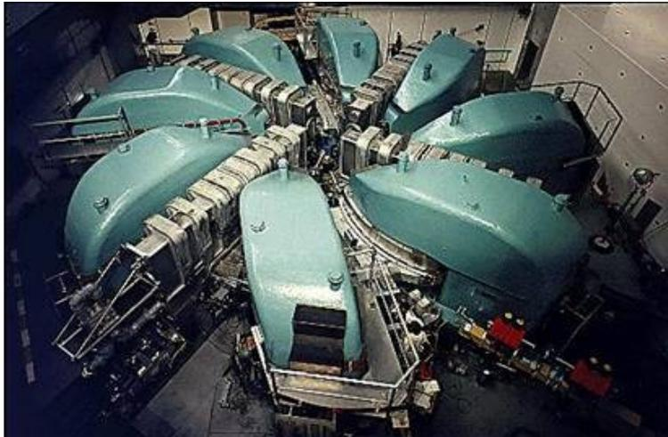
PSI ring cyclotron accelerates  $\sim 10^{16}$  protons per sec to 590 MeV = 0.59 GeV
