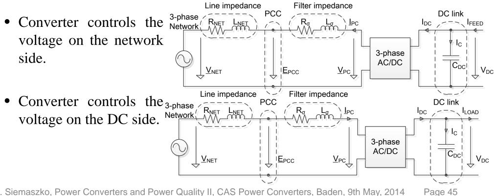
• When voltage unbalance occur, keeping the currents symmetrical has an impact on the instantaneous power.
