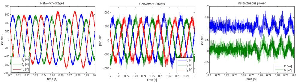
• When the instantaneous power has a second harmonics due to network unbalance, the DC-link voltage will also contain the second harmonic.
