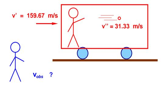
Fling a ball with 31.33 m/s in frame S' moving with 159.67 m/s
