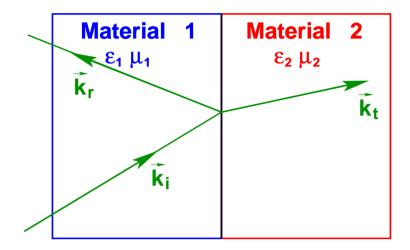
What happens when an incident wave  $(\vec{K_i})$  encounters a boundary between two different media ?
