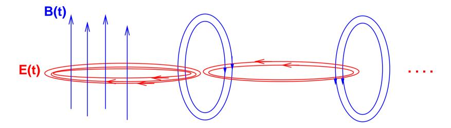
Time varying magnetic fields produce circular electric fields
