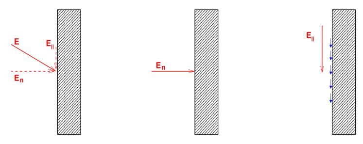
Field parallel to surface  $E_{\parallel}$  cannot exist (it would move charges and we get a surface current):  $E_{\parallel}=0$
