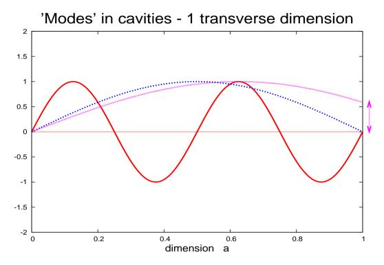
No electric field at boundaries, wave must have "nodes" = zero fields at the boundaries
