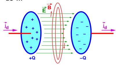
Time varying electric field induces circular magnetic field (using the current density  $\vec{j}_d$ )
