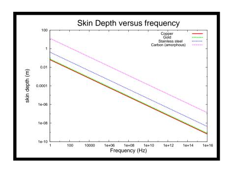
Waves incident on conducting material are attenuated Basically by the Skin depth : (attenuation to 1/e)
