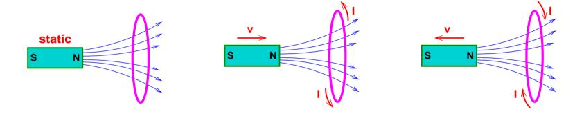
Moving the magnet changes the flux (density or number of lines) through the area  $\implies$
