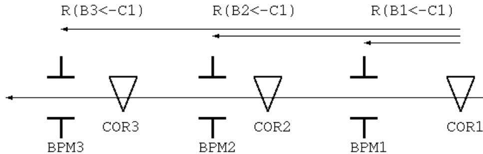
$$\begin{pmatrix} -x_1 \\ -x_2 \\ -x_3 \end{pmatrix} = \begin{pmatrix} R_{12}^{11} & 0 & 0 \\ R_{12}^{21} & R_{12}^{21} & 0 \\ R_{12}^{31} & R_{12}^{32} & R_{12}^{33} \end{pmatrix} \begin{pmatrix} \theta_1 \\ \theta_2 \\ \theta_3 \end{pmatrix}$$
