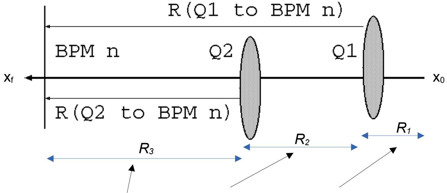
$$\vec{x}_f = R_3 (\vec{q}_2 + R_2) (\vec{q}_1 + R_1) \vec{x}_0$$
