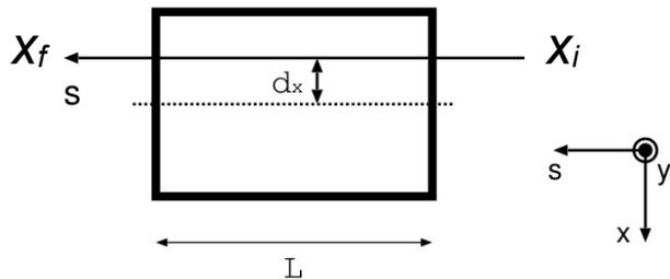
$$\begin{pmatrix} x_f \\ x'_f \end{pmatrix} = \begin{pmatrix} -d_x \\ 0 \end{pmatrix} + \tilde{R} \left[ \begin{pmatrix} d_x \\ 0 \end{pmatrix} + \begin{pmatrix} x_i \\ x'_i \end{pmatrix} \right]$$
