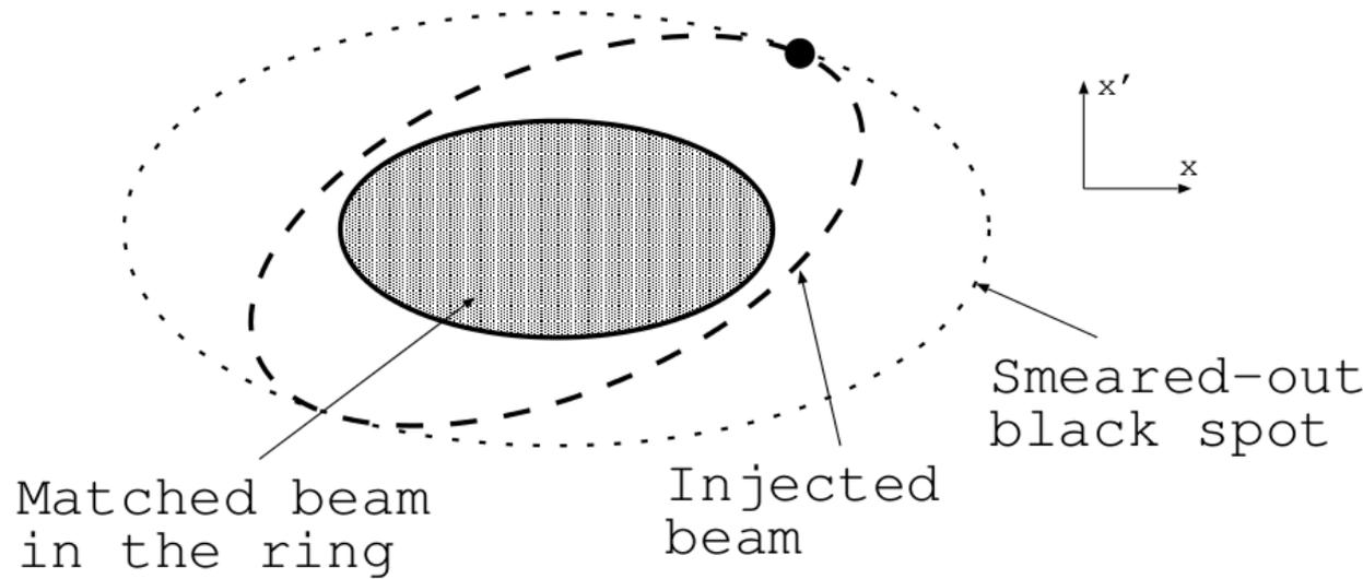
Injecting with transverse offset also leads to filamentation
