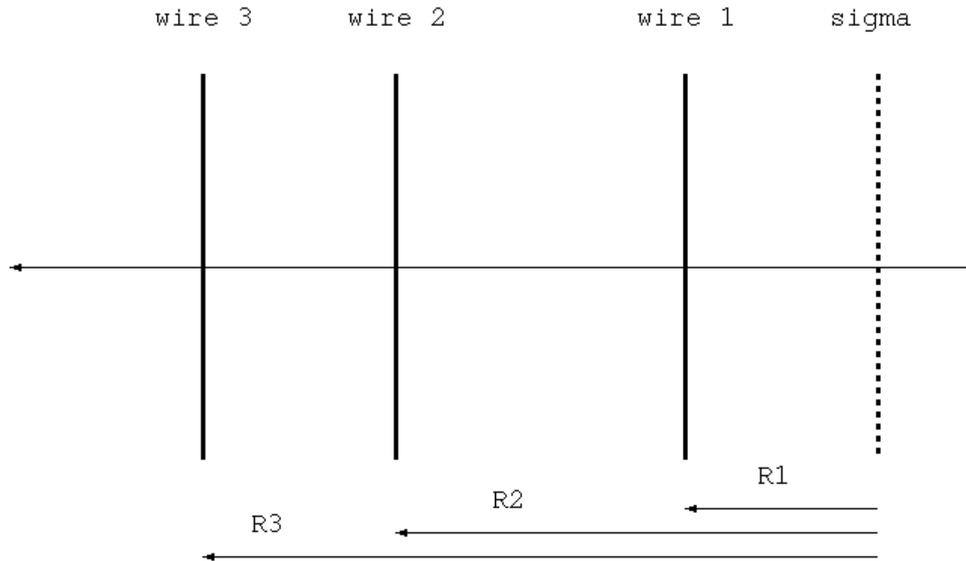
$$\bar{\sigma}_1^2 = (R^1)_{11}^2 \sigma_{11} + 2R_{11}^1 R_{12}^1 \sigma_{12} + (R^1)_{12}^2 \sigma_{22}$$
