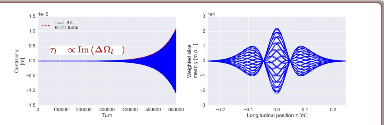
It is to be noted, that these bunch modes are always latently present, but not usually excited. It requires an **impedance as source of energy** together with **chromaticity to generate a synchronization** of the bunch motion with the wake fields kicks in order to **drive a given bunch mode into resonance**.
