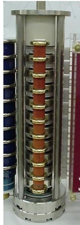
Stack of high-power semiconductor switches (GTOs)
